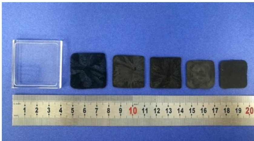
Figure S5. Effect of the PEDOT:PSS to GO weight ratio on the size of the resultant low-profile sponges. From left to right: blank glass mold, PS, PGCS-1, PGCS-2, PGCS-3 and GS.
