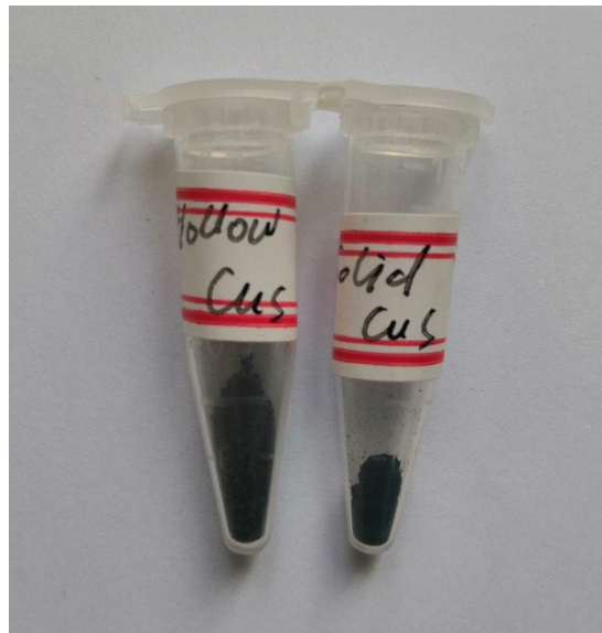
Fig. S2 Hollow CuS nanocube (left) and commercial CuS (right) with the same mass.
