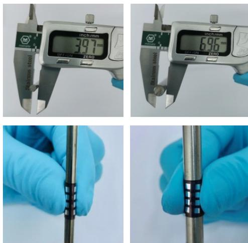
**Figure S8.** The partial image ( $r=2, 3.5$  mm) of bending test and corresponding curved radius.
