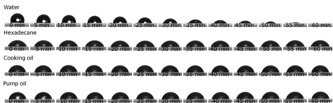
Fig. S4 Images of droplets recorded at various times after their application onto the film
