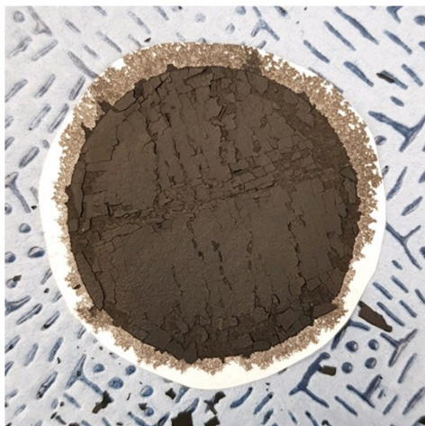
Figure S9. Photograph of the MH paper air cathode without CNFs.
