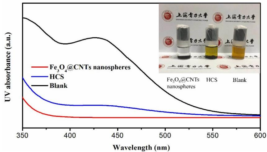
**Fig. S6.** UV-vis absorption spectra of  $\text{Li}_2\text{S}_4$  solution mixed with  $\text{Fe}_3\text{O}_4@\text{CNTs}$  nanospheres and HCS after standing for half an hour
