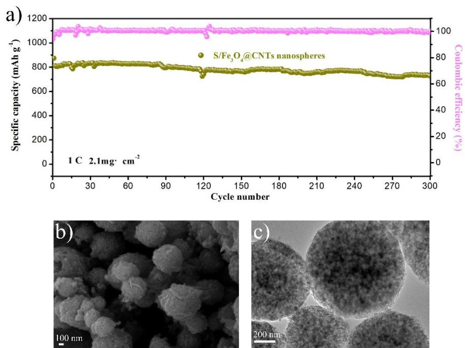
**Fig. S7.** a) Cycling test of the  $\text{S}/\text{Fe}_3\text{O}_4@\text{CNTs}$  nanospheres at 2 C over 300 cycles
