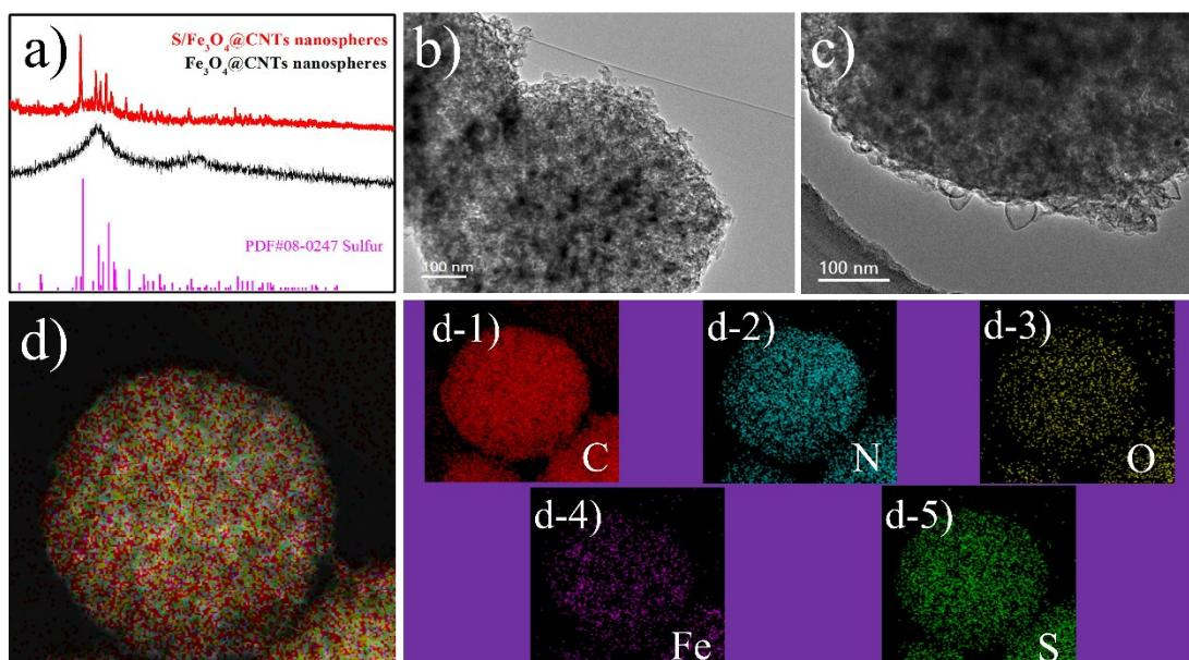
**Fig. S1. Morphology and composition characterizations of S/Fe<sub>3</sub>O<sub>4</sub>@CNTs nanospheres composites:** a) XRD pattern, (b,c) TEM images and (d) corresponding elemental mappings of the S/Fe<sub>3</sub>O<sub>4</sub>@CNTs nanospheres composites.
