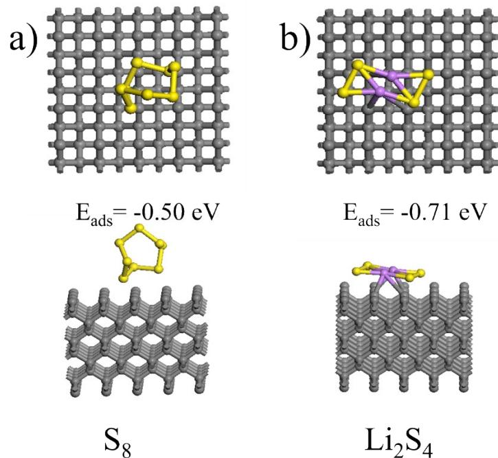
**Fig. S8. binding geometric configurations and binding energies of  $\text{S}_8$  and  $\text{Li}_2\text{S}_4$  species with graphene**
