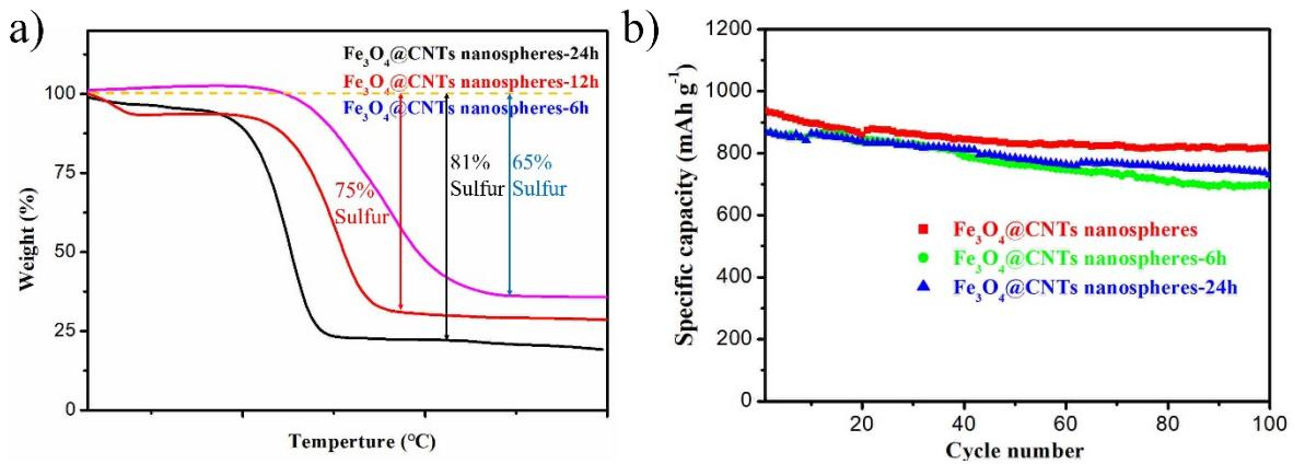
**Fig. S4.** a) TG curves of S/ $\text{Fe}_3\text{O}_4$ @CNTs nanospheres-6 h, S/ $\text{Fe}_3\text{O}_4$ @CNTs nanospheres-12 h, and S/ $\text{Fe}_3\text{O}_4$ @CNTs nanospheres-24 h b) Corresponding cyclic performance at 1C over 100 cycles with 2.1 mg cm<sup>-2</sup> sulfur loading
