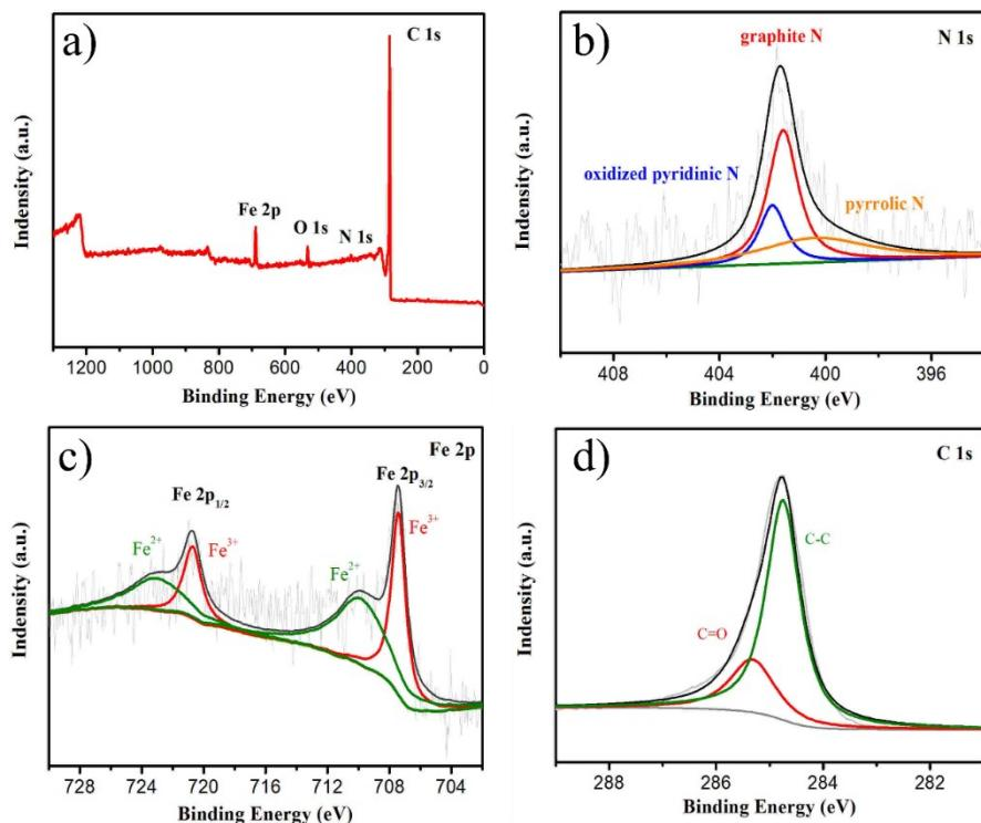
**Fig. S5.** (a) XPS spectra of  $\text{Fe}_3\text{O}_4$ @CNTs nanospheres; and (b-d) the high resolution XPS spectra of N 1s, C 1s, and Fe 2p
