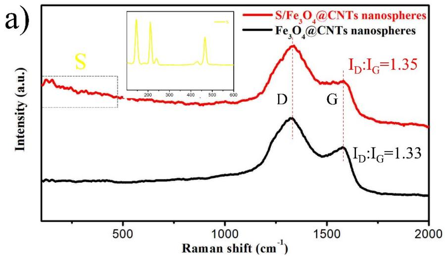
**Fig. S2. a)** Raman spectra of  $\text{Fe}_3\text{O}_4@\text{CNTs}$  nanospheres and  $\text{S}/\text{Fe}_3\text{O}_4@\text{CNTs}$  nanospheres
