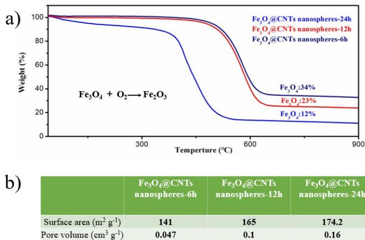
**Fig. S3. a)** TGA curve of  $\text{Fe}_3\text{O}_4@\text{CNTs}$  nanospheres in air; b) surface area and pore volume of the  $\text{Fe}_3\text{O}_4@\text{CNTs}$  nanospheres-6 h,  $\text{Fe}_3\text{O}_4@\text{CNTs}$  nanospheres-12 h and  $\text{Fe}_3\text{O}_4@\text{CNTs}$  nanospheres-24 h
