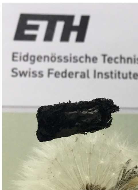
Fig. S5 Photograph of a monolithic N-rGO foam on a dandelion flower, illustrating the low density of the foam.
