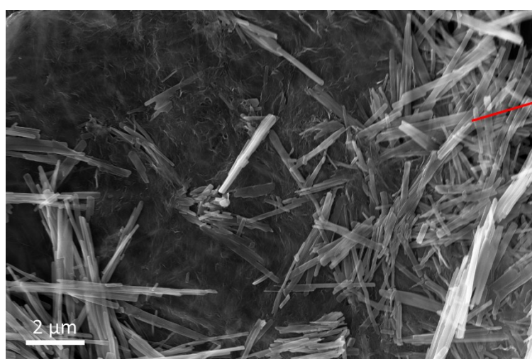
Fig. S4 SEM overview image of NVO@rGO with NVO nanobelts well embedded in the rGO network and with NVO nanobelts less closely connected to the rGO sheets.
