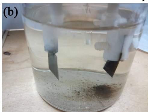
Fe 2 O 3 /CC After 10000 cycles Mxene@Fe 2 O 3 /CC After 10000 cycles
