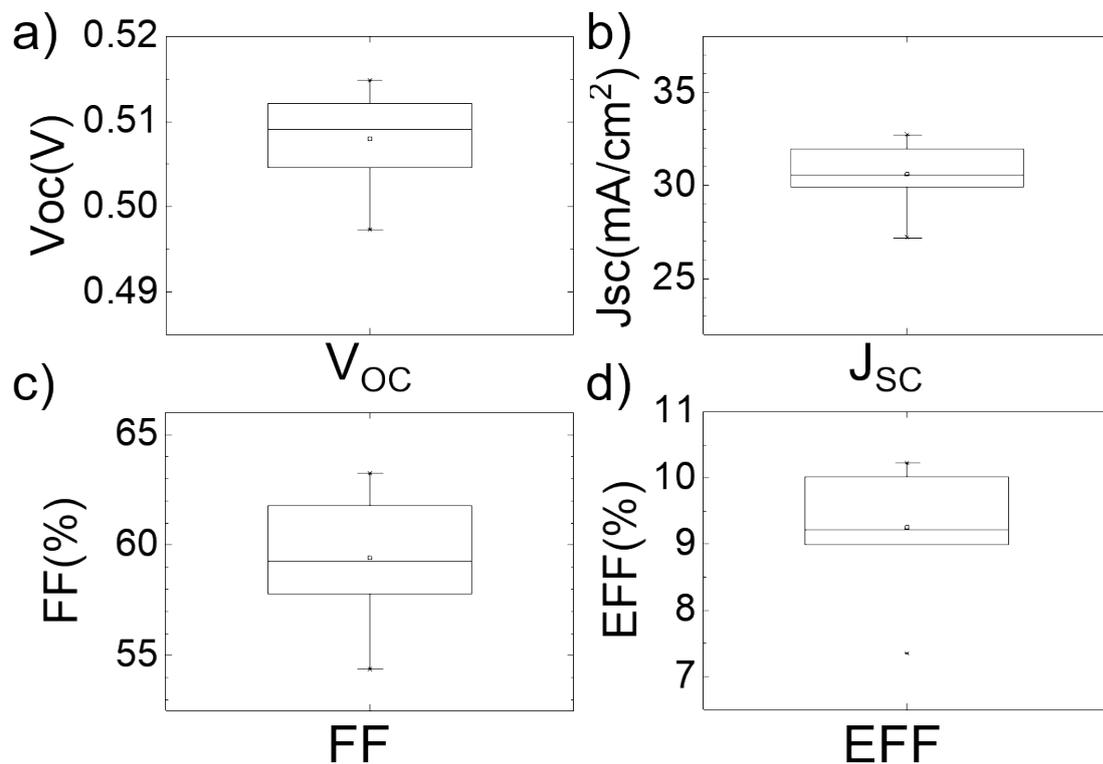
**Supplementary Fig. S5** The statistics of (a) V<sub>OC</sub>, (b) J<sub>SC</sub>, (c) FF, and (d) EFF from the *J-V* curve of 8 CZTSSe solar cells on SS foil. The best cell was certified by KIER (supplementary Fig. S1).
