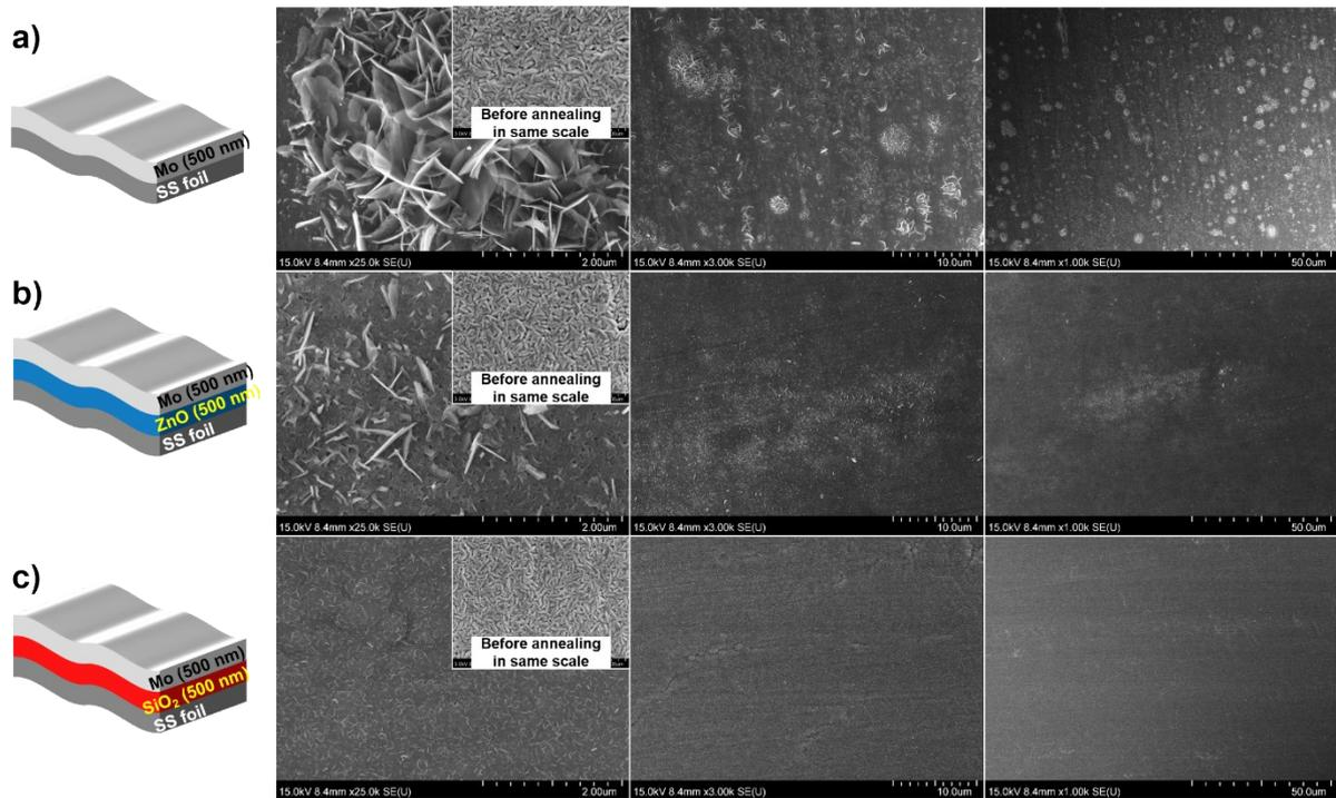
**Supplementary Fig. S2** SEM images of the Mo back contact layer surfaces for various diffusion barriers. (a) Mo/SS foil structure, (b) Mo/ZnO/SS foil structure, and (c) Mo/SiO<sub>2</sub>/SS foil structure after annealing at 800 °C for 1 hr.
