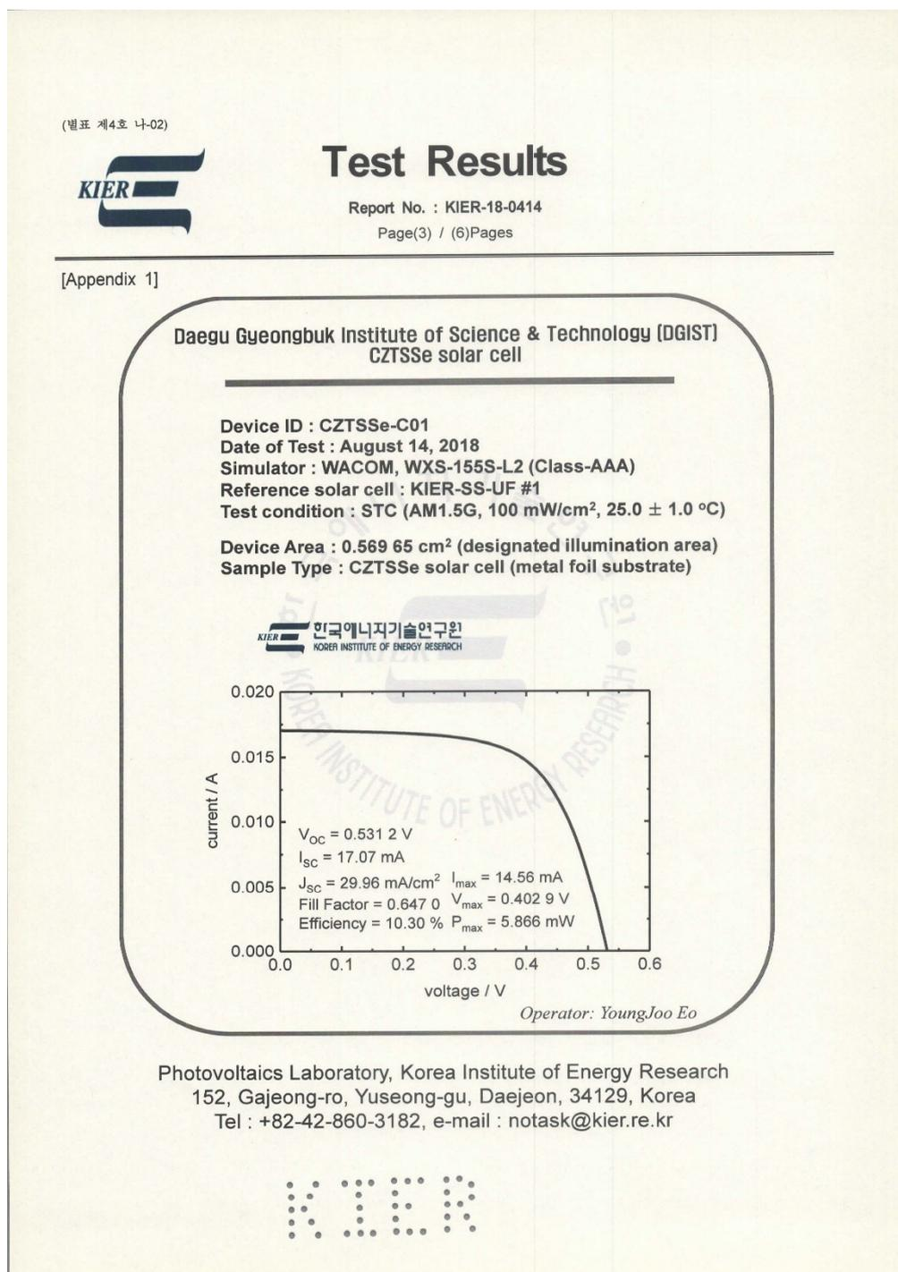
Supplementary Fig. S1 The  $J$ - $V$  curve of the recording device from KIER.
