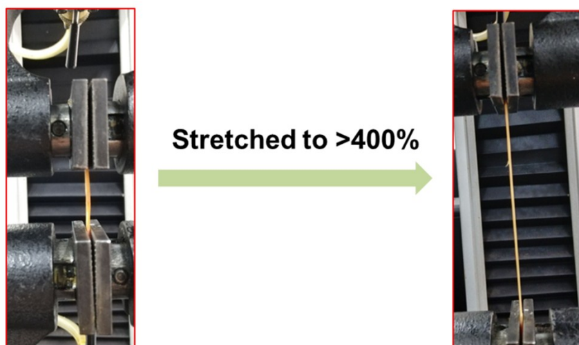
Fig. S3 Photographic images of a DC-PCM8K film before and after stretching.
