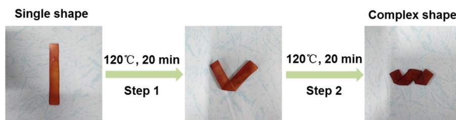
Fig. S4 The complex shape of DC-PCM8K can be achieved from single shape through two-step reshaping process, which indicates that the solid-state plasticity show a cumulative effect.
