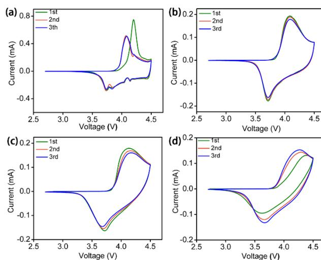
Fig. S6 CV of (a) liquid electrolyte-based LiCoO<sub>2</sub> battery, ASSLBs with (b) bare LiCoO<sub>2</sub>, (c) LiCoO<sub>2</sub> particles coating and (d) LiCoO<sub>2</sub> electrode coating. All batteries were tested at 60°C.
