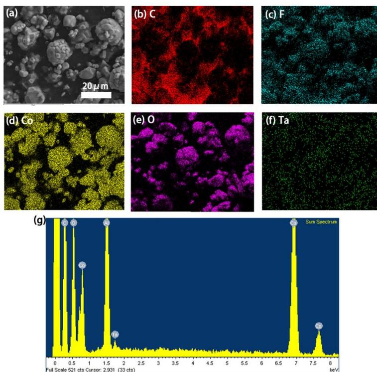
Fig. S5 SEM image and EDX mappings of the electrode with ALD LTO coated LiCoO<sub>2</sub> particles. (a) SEM image; EDX mappings of (b) C, (c) F, (d) Co, (e) O, and (f) Ta elements. (g) Corresponding EDX spectrum.
