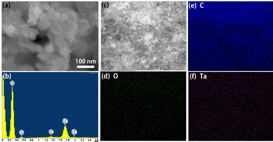
Fig. S9 (a) SEM image of carbon black particles with ALD-LTO coating. (b) EDX spectrum of carbon black particles with ALD-LTO coating; (c) corresponding SEM image of EDX mapping area; (d) corresponding O distribution; (e) corresponding C distribution; (f) corresponding Ta distribution.
