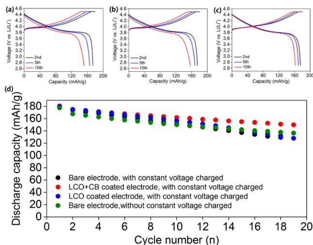
Fig. S14 Charge/discharge profiles of ASSLBs with (a) bare LiCoO<sub>2</sub> electrode, (b) LCO-coating protection electrode, and (c) LCO+CB-coating protection electrode at 0.2 C and 60 oC with constant voltage charge step. (d) Comparison of discharge capacity of ASSLBs with different electrodes.
