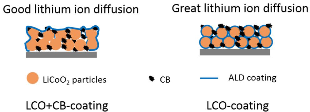
Fig. S8 Comparison of ALD coating in LCO+CB-coating electrode and LCO-coating electrode. A better lithium ion diffusion can be achieved in LCO-coating electrode.
