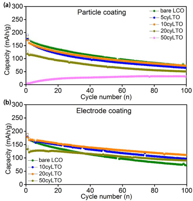
Fig. S7 The influences of ALD coating thickness on the performances of ASSLBs with (a) particles coating and (b) electrode coating.
