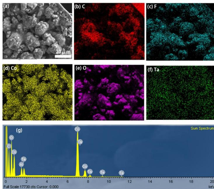
Fig. S4 SEM image and EDX mappings of ALD LTO coated LiCoO<sub>2</sub> electrode. (a) SEM image; EDX mappings of (b) C, (c) F, (d) Co, (e) O, and (f) Ta elements. (g) Corresponding EDX spectrum.
