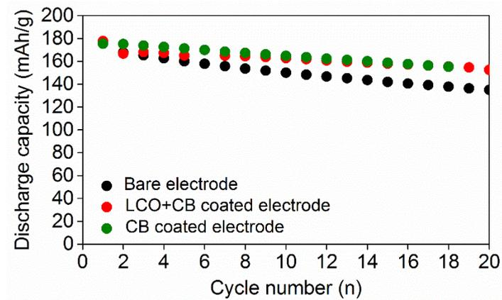
Fig. S10 Comparison of cycling performance of the ASSLBs with bare  $\text{LiCoO}_2$  electrode, LCO+CB coated electrode and CB coated  $\text{LiCoO}_2$  electrode.
