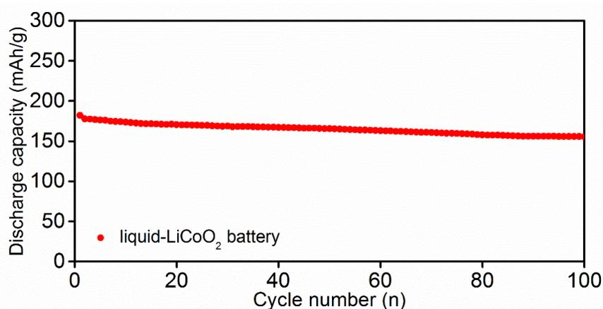
Fig. S12 Cycling performance of  $\text{LiCoO}_2$  battery with carbonate-based liquid electrolyte. The charge/discharge voltage window is from 2.7 – 4.5 V. The stable performance indicates the  $\text{LiCoO}_2$  particles are stable. The protection may not be so critical for performance enhancement. Thus, the capacity decay of the  $\text{LiCoO}_2$  ASSB is the contribution of the decomposition of SPE.
