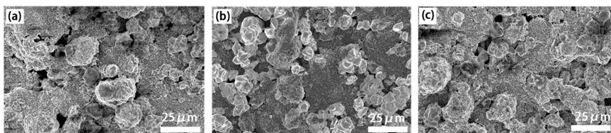
Fig. S1 SEM images of (a) bare LCO electrode, (b) electrode with ALD LTO coated LiCoO<sub>2</sub> particles (LCO-coating protection) and (c) ALD LTO coated electrode (LCO+CB-coating protection).
