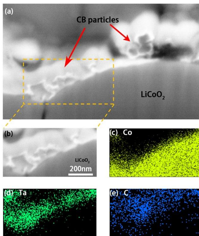
Fig. S3 (a) Cross-section view of SEM image of LiCoO<sub>2</sub> particle covered with carbon black particles with LTO coating. (b) The selected area for EDX mapping and its corresponding element distribution of (c) Co, (d) Ta, (e) C.
