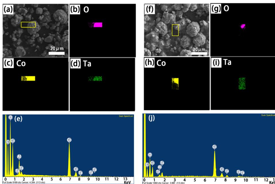
Fig. S2 (a) SEM image and EDX mappings of selected area for electrode with 50 cycles ALD LTO coated LiCoO<sub>2</sub> particles (LCO-coating protection) and its corresponding (b)
