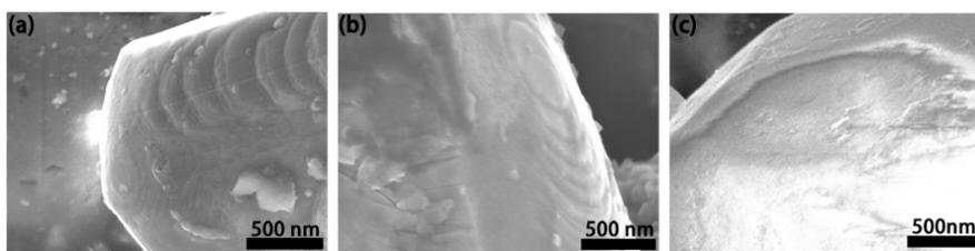
Fig. S13 SEM images of LiCoO<sub>2</sub> particles collected from ASSLBs with (a) bare electrode, (b) LCO-coating protection, and (c) LCO+CB-coating protection after 200 cycles.
