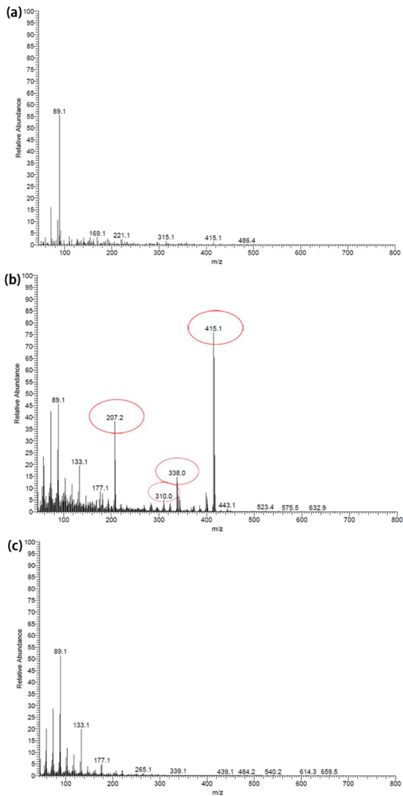
Fig. S11 The mass spectrometry (MS) results. (a) Pristine PEO-based SPE. (b) PEO-carbon composite after charging to 4.5 V and holding for 20 h; the red circles point out the signals related to the decomposition of PEO-based SPE. (c) PEO-ALD LTO carbon
