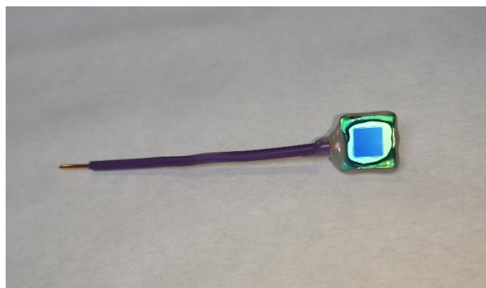
Fig. S. 1: p + n-Si photoanode, where a 0.5 cm 2 active area (darker region) was lithographically defined by SiO 2 passivation on a silicon n-type wafer (0.1-0.5 ohm.cm resistivity), ALD-protected and further Ag paint soldered to a Cu wire and isolated with thermoplastic.
