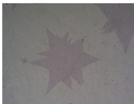
Fig. S7 Transferred monolayer dendritic \text{MoS}_2 flakes on glassy carbon.
