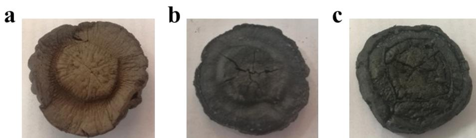
**Figure S5.** Photographs of the carbonized carrots. a) The pyrolysis temperature of 300 °C with the ethanol treatment. b) The pyrolysis temperature of 550 °C without the ethanol treatment. c) The pyrolysis temperature of 550 °C with the ethanol treatment.
