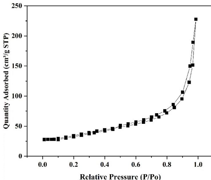
**Fig. S1** Nitrogen adsorption–desorption isotherms of LD-graphene aerogel.
