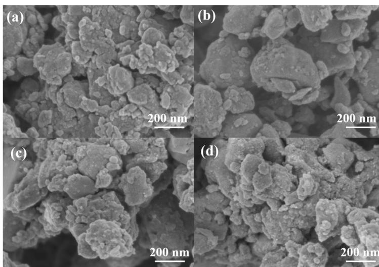
**Fig. S4** SEM images for solid product from biomass pyrolysis: (a) rice husk; (b) rice straw; (c) cornstalk and (d) poplar wood.
