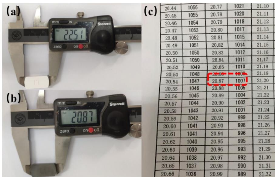
**Fig. S2** (a) Original length of alumina temperature measuring cuboid; (b) length of alumina temperature measuring cuboid after the heating process is finished; (c) standard data table for the alumina temperature measuring cuboid.
