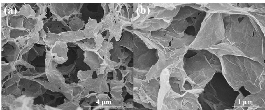
**Fig. S3** SEM images of LD-graphene aerogel after several times of microwave-assisted pyrolysis reactions.
