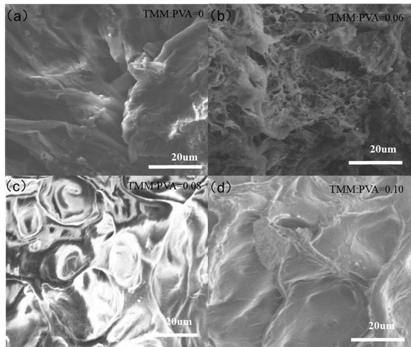
Fig.S3 SEM images of pure PVA film and the TMM cross-linked PVA film at different molar fractions.
