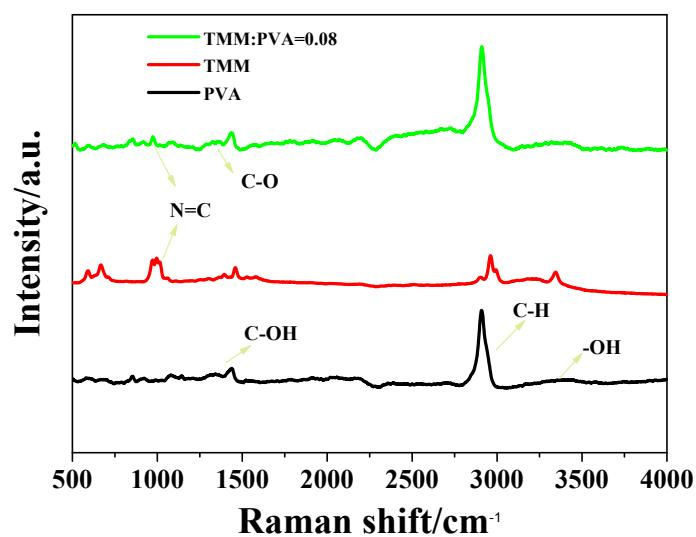
Fig. S4 Raman spectrum for pure PVA ,crosslinking agent TMM and the TMM functionalized PVA at 0.08 molar fraction.
