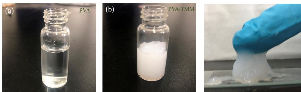
Fig. S2 The photographs of the pure PVA solution and the cross-linked PVA gel at 0.08 molar fraction of TMM.
