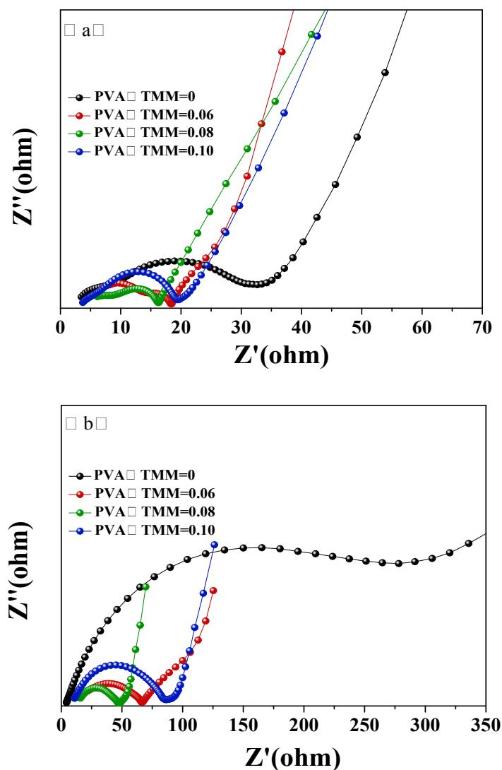
Fig. S7 Nyquist plots for of the Si electrodes using PVA binder at different TMM molar fractiona (a) after rate test and (b) after 500 charge-discharge cycles.
