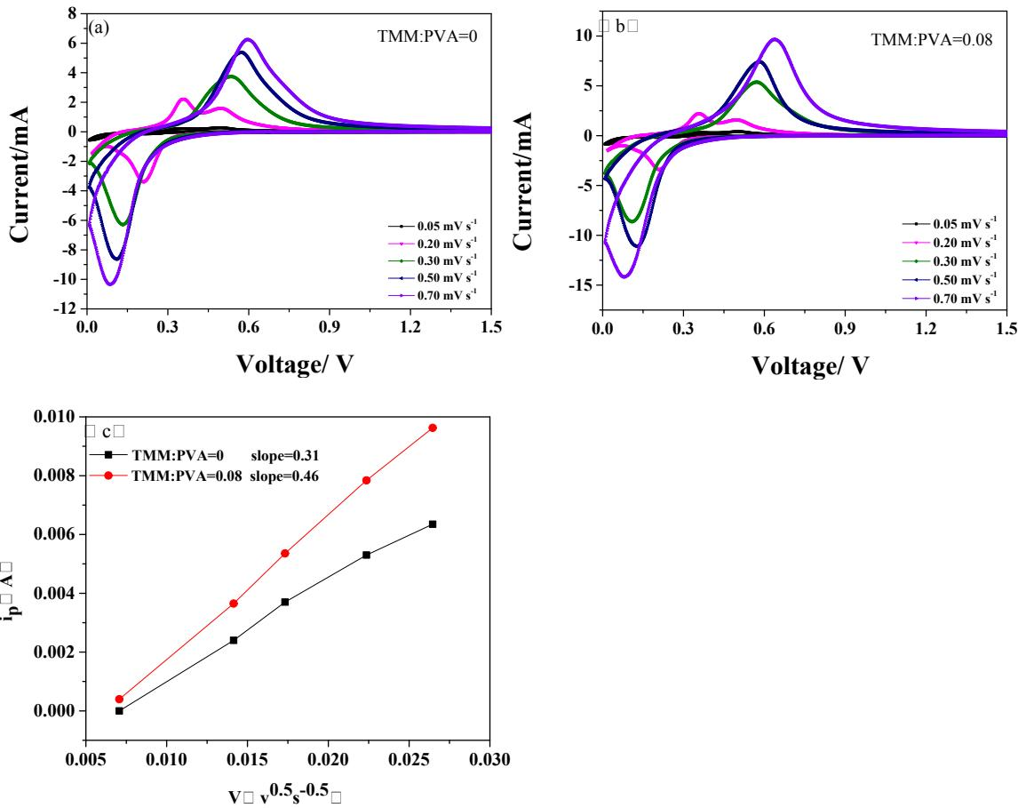
Fig. S6. The cyclic voltammetry (CV) curves of the Si electrodes using PVA binder (a) without and (b) with 0.08 molar fraction of TMM cross-linker at different scan rates and (c) the fit between square root of scan rate and anodic peak current.
