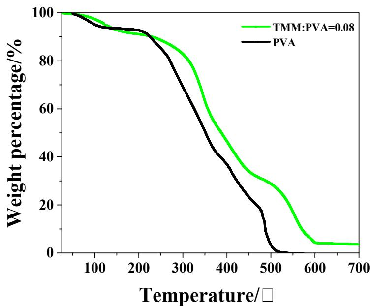
Fig. S5 TG diagram for pure PVA and the TMM functionalized PVA at 0.08 molar fraction.
