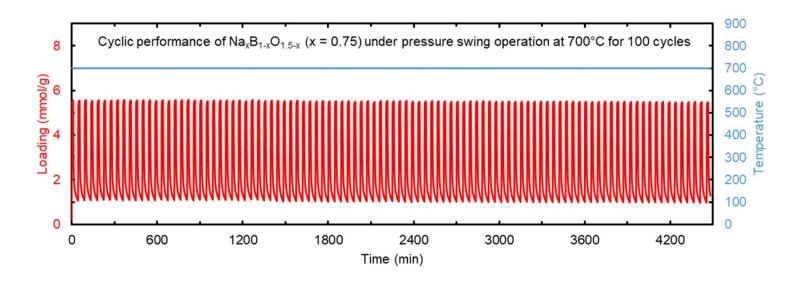
Figure S1. Cyclic regenerability of  $CO_2$  uptake and the desorption by  $Na_xB_{1-x}O_y$  (x=0.75) up to 100 cycles by pressure swing operation on repeated switching of the gas stream between 100%  $CO_2$  (p $CO_2$  = 1 bar) and 100%  $N_2$  (p $CO_2$  = 0 bar) at 700°C.
