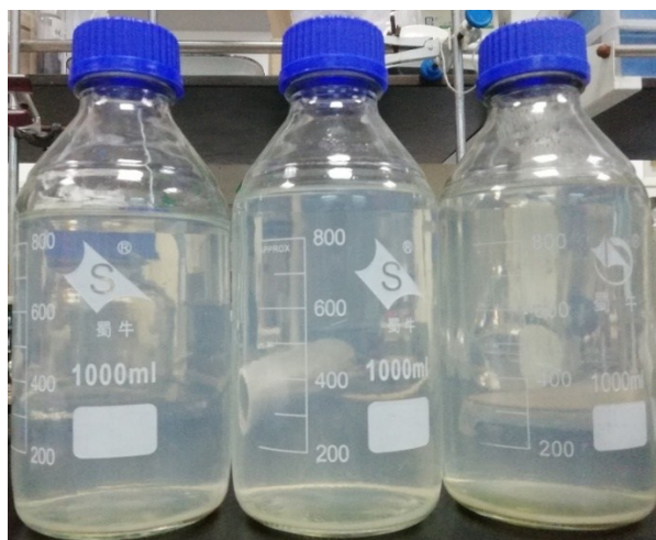
Fig. S6 A photo of vermiculite nanosheets suspensions after 25 months. A nearly transparent vermiculite nanosheets dispersion with a concentration of 1 \text{ mg mL}^{-1} was obtained after removing the unexfoliated vermiculite flakes by centrifugation at 10000 r.p.m. for 20 min. The vermiculite nanosheets suspensions can keep stable and no appreciable precipitation was found even after 25 months.
