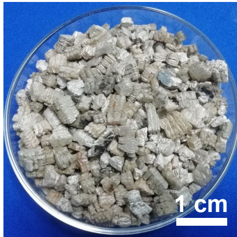
Fig. S1 A photo of thermally expanded vermiculite powders. The particle size of silvery white vermiculite powders is about 8-13 \mu\text{m} .
