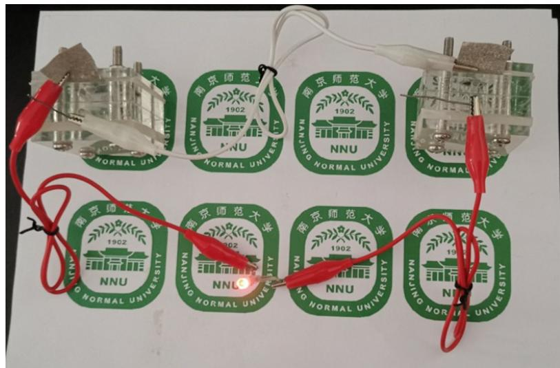
**Fig. S11.** A LED lamp ( $\sim 3.0$  V) could be powered up by two Zn-air batteries in series with the NiCoFeP-HN + Pt/C catalyst as air-cathode.
