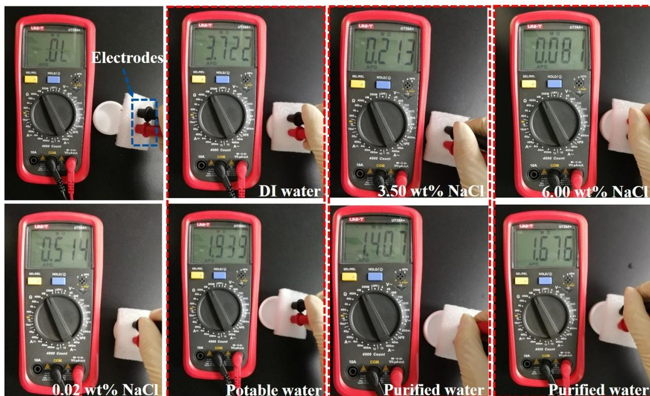
Figure S15. Evaluation of water purity using a multimeter with a constant distance between electrodes.
