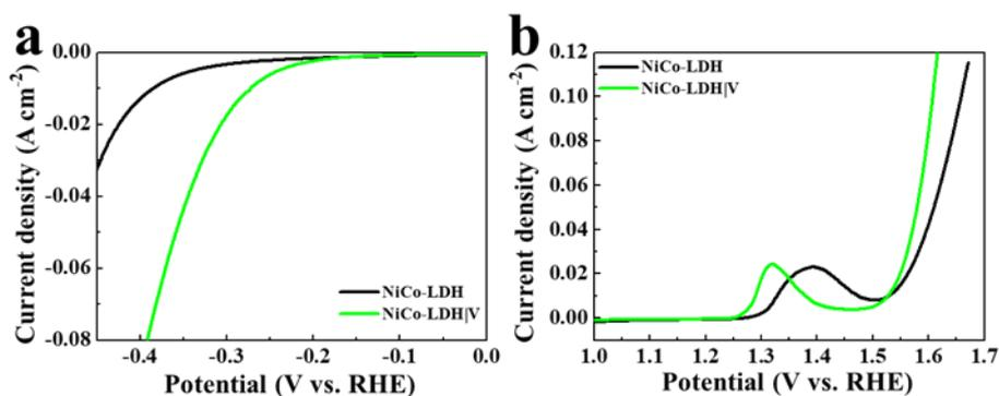
**Fig. S7** The comparison of (a) HER and (b) OER polarization curves between NiCo-LDH and NiCo-LDH|V.
