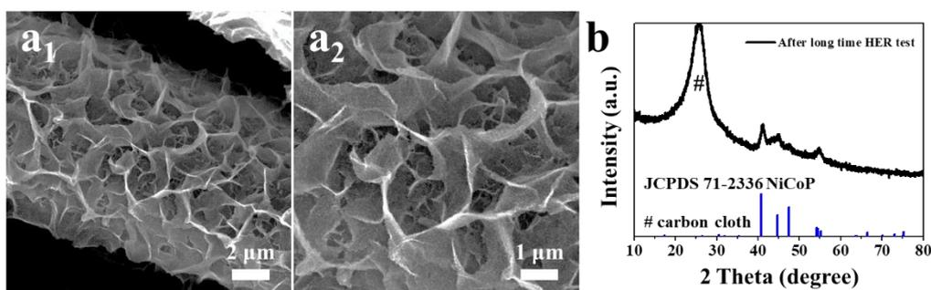
**Fig. S9** (a) SEM images, (b) XRD pattern of Ar-NiCoP|V after long time HER test.
