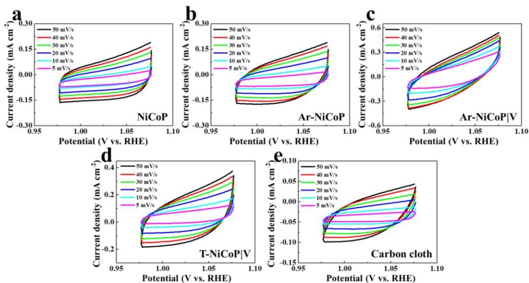
**Fig. S13** CV curves of obtained samples for estimating the  $C_{dl}$  in OER tests.
