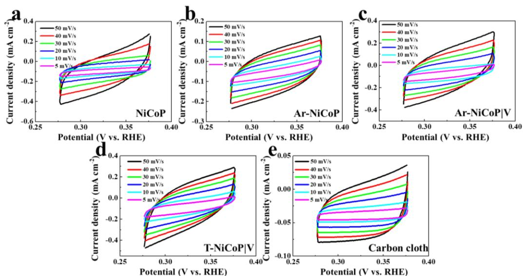
**Fig. S8** CV curves of obtained samples for estimating the  $C_{dl}$  in HER tests.
