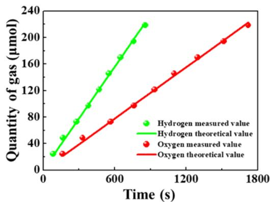
**Fig. S17** Amounts of gas calculated and experimentally measured along reaction time for overall water splitting. The theoretical line represents the amount of H<sub>2</sub> or O<sub>2</sub> expected for a 100% Faraday efficiency
