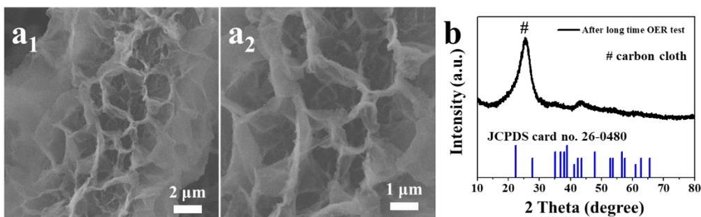
**Fig. S14** (a) SEM images, (b) XRD pattern of Ar-NiCoP|V after long time OER test.
