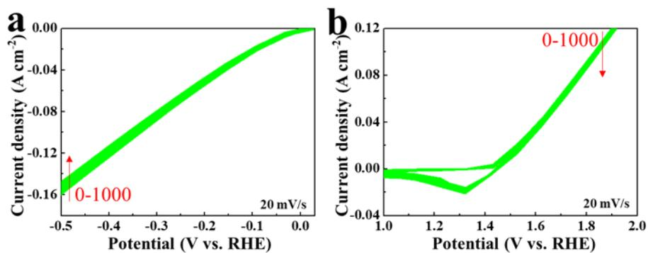
**Fig. S11** The (a) HER and (b) OER cyclic voltammetry curves of 1000 cycles.
