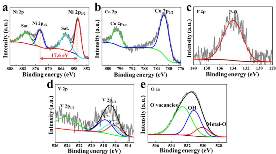
**Fig. S16** XPS (a) Ni 2p, (b) Co 2p, (c) P 2p, (d) V 2p and (e) O 1s spectra of Ar-NiCoP|V after 1000 cycles in OER tests
