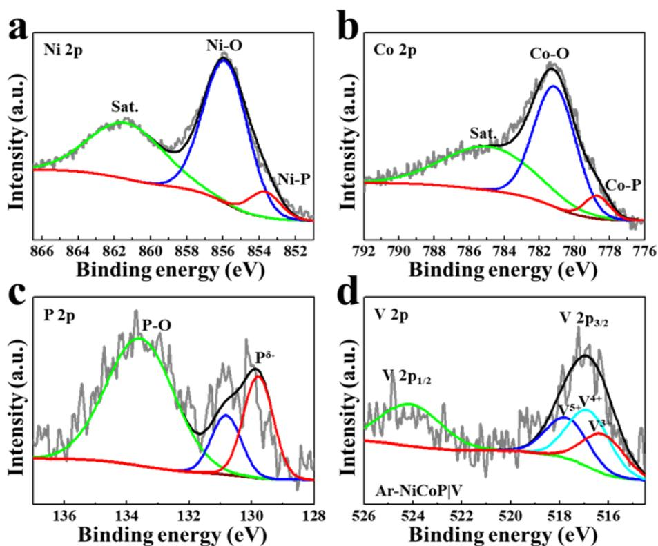
**Fig. S12** XPS (a) Ni 2p, (b) Co 2p, (c) P 2p and (d) V 2p spectra of Ar-NiCoP|V after 1000 cycles in HER tests
