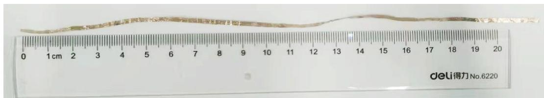
Fig. S2. A photograph of the obtained flexible bulk nanoporous  $\text{AuCu}_3@\text{Au}$  electrode.
