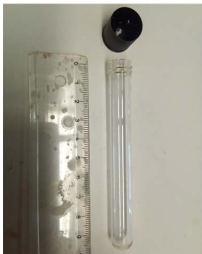
Fig. S1. Tube used in the photocatalytic experiments in this work (left). Emission spectrum of the LED module (filled) and transmission of the glass tube used for photocatalytic tests (black line) (right).
