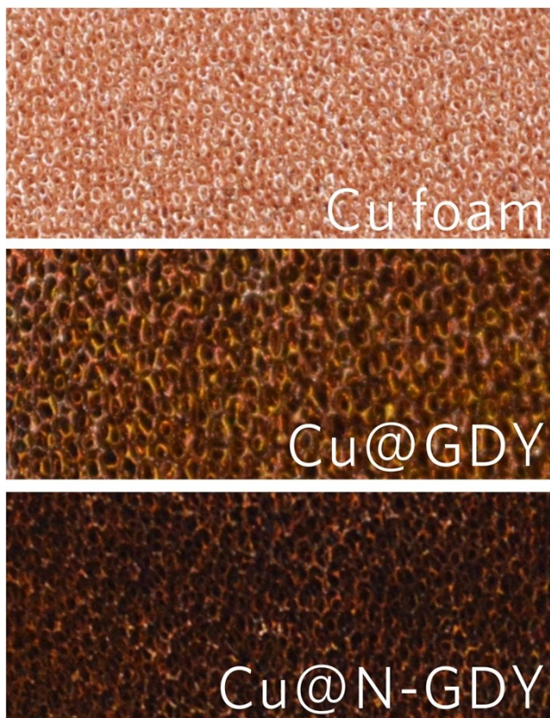
Fig. S3. Digital photographs of the pristine Cu foam, GDY host after the low-temperature wet-chemistry synthesis, and N-GDY host after the thermal nitridation process.
