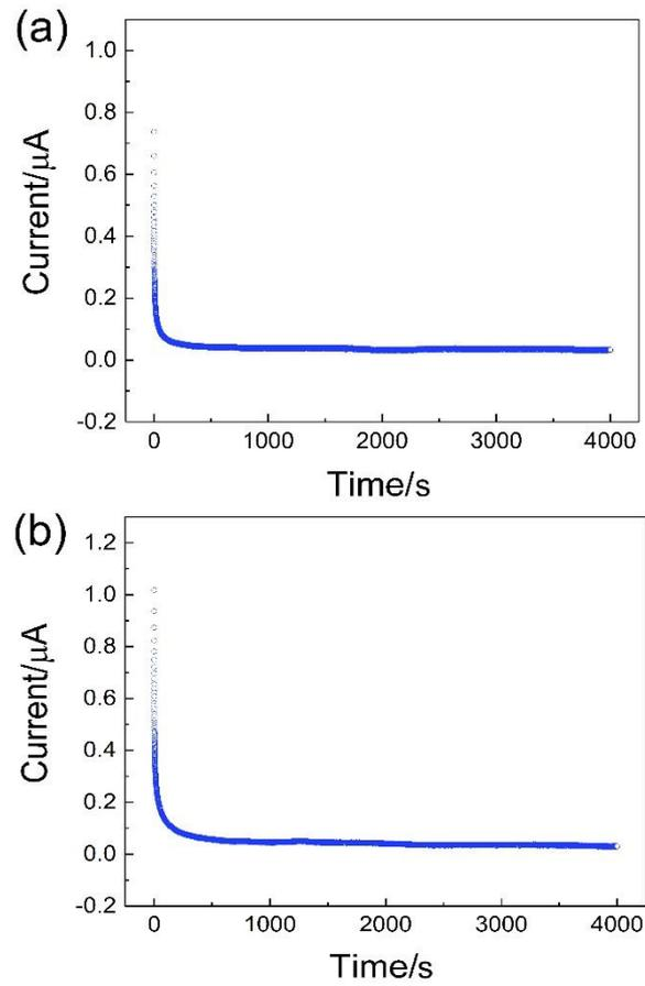
**Figure S4.** DC polarization curves of the polymerized electrolytes based on stainless steel/electrolyte/stainless steel symmetric cells. (a) Polymerized composite electrolytes with 10% LLZO, (b) polymerized polymer electrolytes without LLZO fillers.
