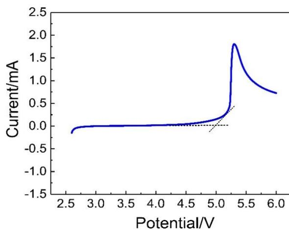
**Figure S6.** LSV curves of the polymer electrolyte without LLZO fillers.
