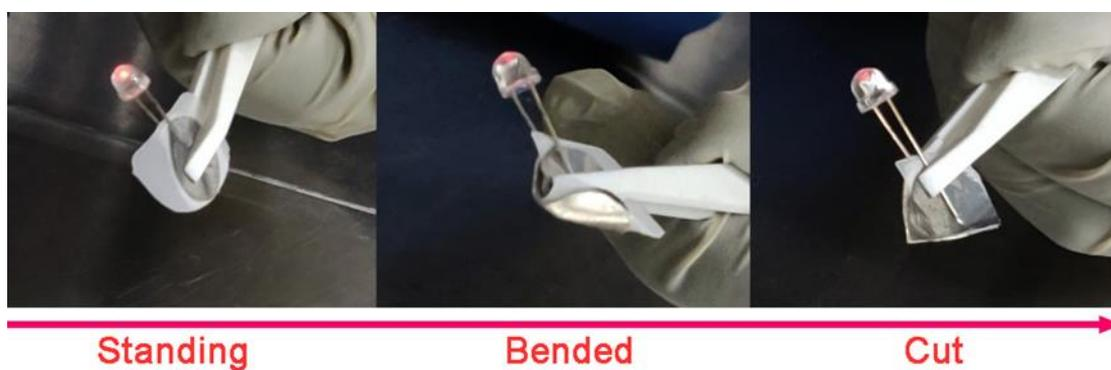
**Figure S14.** Safety evaluation of solid-state battery Li/PCE-10/NCM622 under destructive conditions: standing, bended, and cut.
