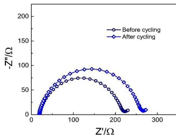
**Figure S7.** Impedance spectra of the Li/PCE-10/Li symmetric cell before and after 500 cycles at a current density of  $0.5 \text{ mA cm}^{-2}$ .
