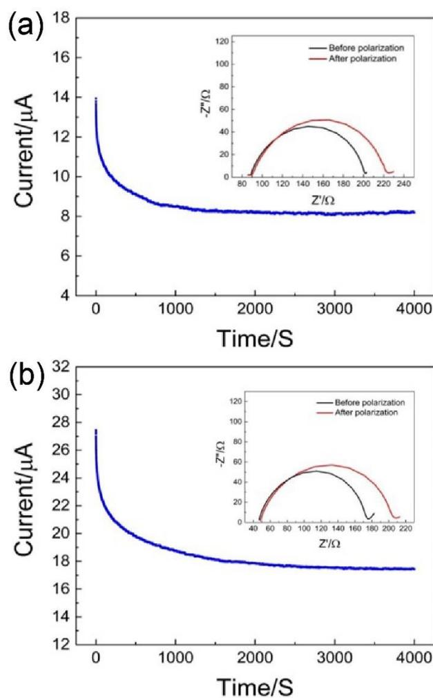
**Figure S5.** DC polarization curves of the polymerized electrolytes based on Li/electrolyte/Li symmetric cells. Insets: impedance spectra of the cells before and after polarization. (a) Polymerized composite electrolytes with 10% LLZO, (b) polymerized polymer electrolytes without LLZO fillers.
