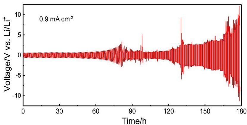
**Figure S9.** Voltage profiles of the Li/PCE-10/Li symmetric cell at a current density of  $0.9 \text{ mA cm}^{-2}$ .
