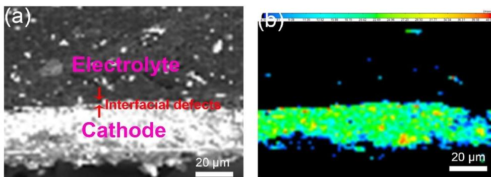
**Figure S10.** (a) EPMA image, and (b) WDS mapping of the interface between the cathode and the ex-situ polymerized composite electrolyte.
