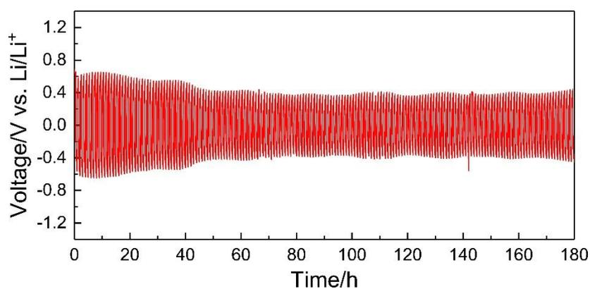
**Figure S8.** Voltage profiles of the Li/PCE-10/Li symmetric cell at a current density of  $0.6 \text{ mA cm}^{-2}$ .
