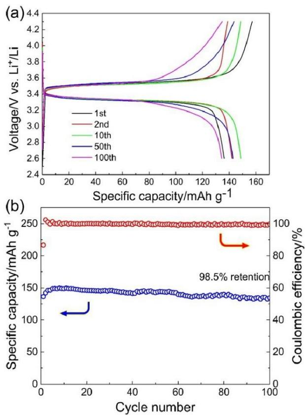
**Figure S15.** (a) Typical charge/discharge profiles, and (b) cycling stability and Coulombic efficiency of Li/PCE-10/LiFePO<sub>4</sub> solid-state battery in the voltage range of 2.6 to 4.3 V under 0.2 C.
