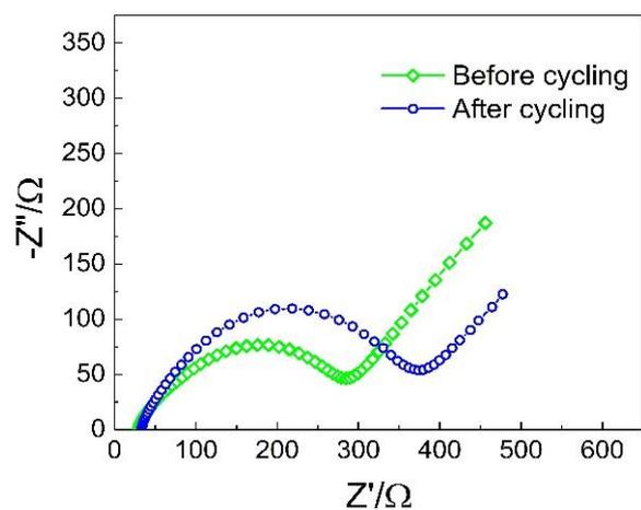
**Figure S12.** Impedance spectra of the Li/PCE-10/NCA battery before and after cycling at a rate of 0.3 C.
