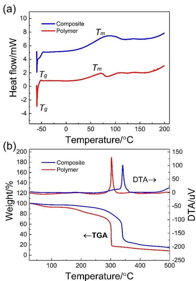
**Figure S3.** Thermal performances of the polymerized electrolytes (polymer and composite electrolytes): (a) DSC curves, (b) TG-DTA curves.
