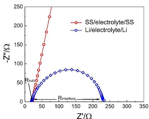
**Figure S11.** Impedance spectra of PCE-10 with blocking electrodes (stainless steel, SS) and reversible electrodes (metallic Li).
