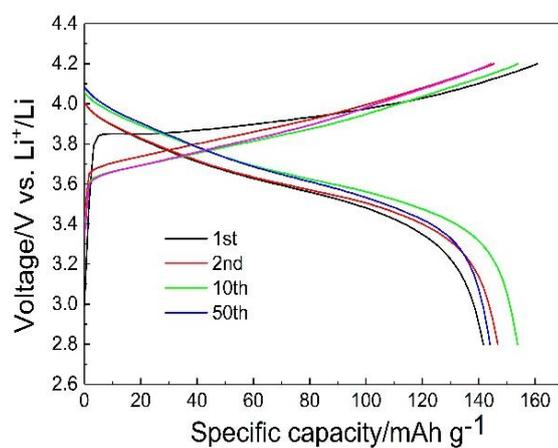
**Figure S13.** Typical charge/discharge profiles of Li/PCE-10/NCM622 solid-state battery in the voltage range of 2.8 to 4.2 V under 0.5 C.
