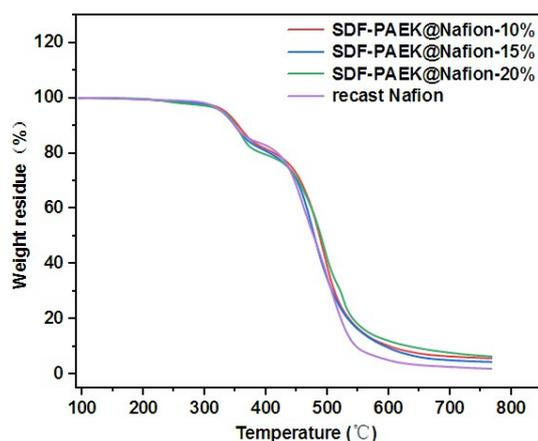
Figure S2. TGA curves of recast Nafion membrane and composite membranes.
