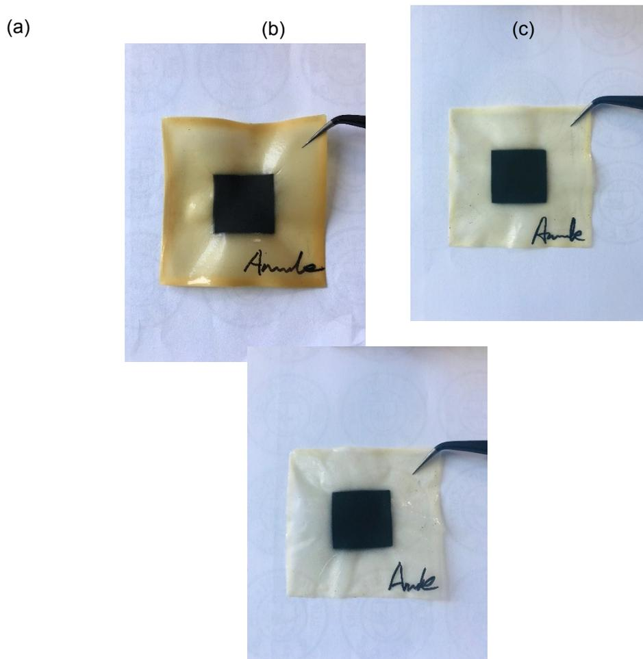
Figure S4. Photographs of composite membranes: SDF-PAEK@Nafion-20% (a); SDF-PAEK@Nafion-15% (b); SDF-PAEK@Nafion-10% (c).
