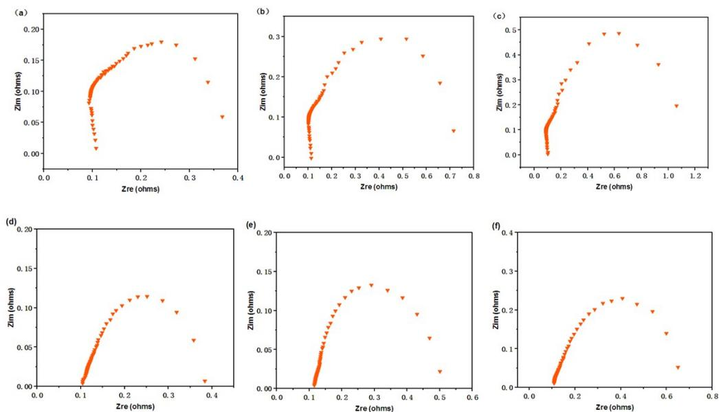
Figure S5. Nyquist plots of SDF-PAEK@Nafion-15% single cells impedance spectra. 1M: (a), (b), and (c); 2M: (d), (e), and (f).
