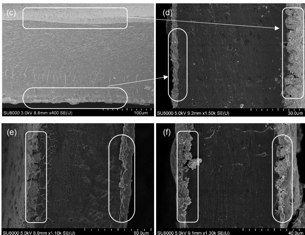
Figure S3. Cross-sectional SEM imagines of (a), (b) SDF-PAEK@Nafion-15%; (c) SDF-PAEK@Nafion-15% with catalyst; (d) SDF-PAEK@Nafion-15% with catalyst after single-cell test, (e) SDF-PAEK@Nafion-10% with catalyst after single-cell test, (f) SDF-PAEK@Nafion-20% with catalyst after single-cell test.
