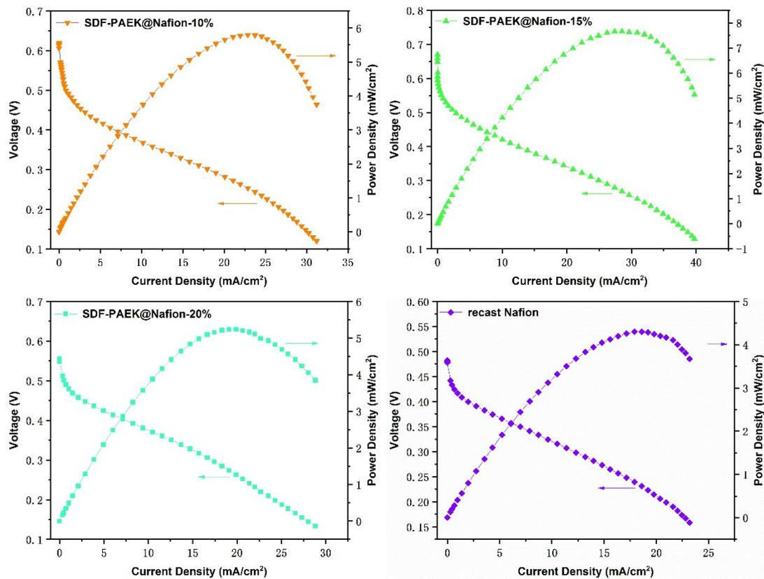
Figure S6. The polarization and power density curves of membranes at 2 M methanol solution at 25 °C.
