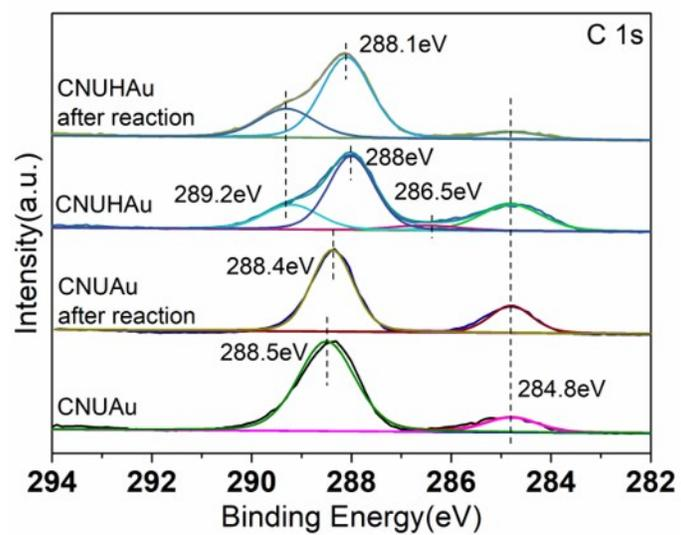
Figure S7. C 1s XPS spectra for CNUAu and CNUHAu before and after reaction
