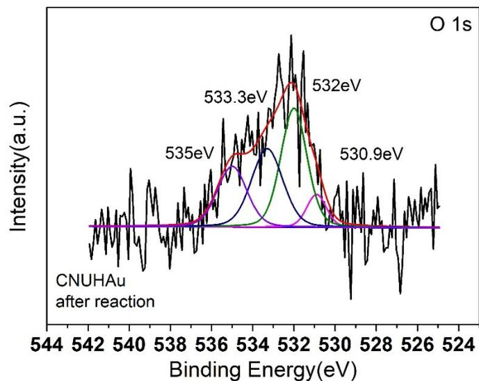
Figure S5. The O 1s XPS spectrum of CNUHAu after photocatalytic test
