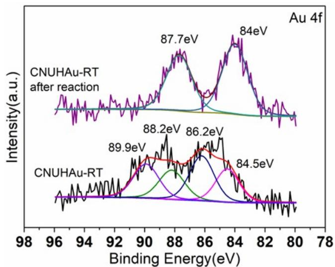
Figure S6. Au 4f XPS spectra for CNUHAu-RT sample before and after reaction
