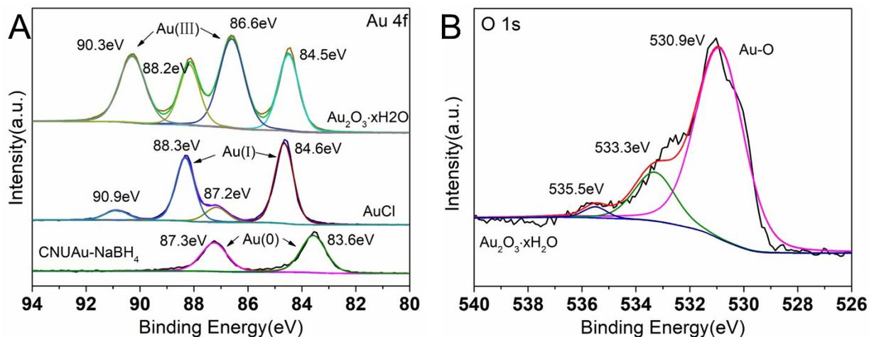
Figure S2. (A) Au 4f XPS spectra of CNUAu-NaBH<sub>4</sub>, AuCl and Au<sub>2</sub>O<sub>3</sub>·xH<sub>2</sub>O, (B) O 1s XPS spectra of Au<sub>2</sub>O<sub>3</sub>·xH<sub>2</sub>O
