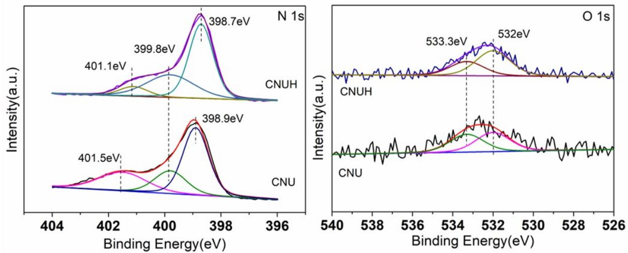
Figure S3. N 1s and O 1s XPS spectra for CNU and CNUH
