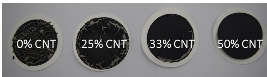
Fig. S4. Digital photos of SWCNT/rGO with different content of SWCNT on PVDF filtration paper.
