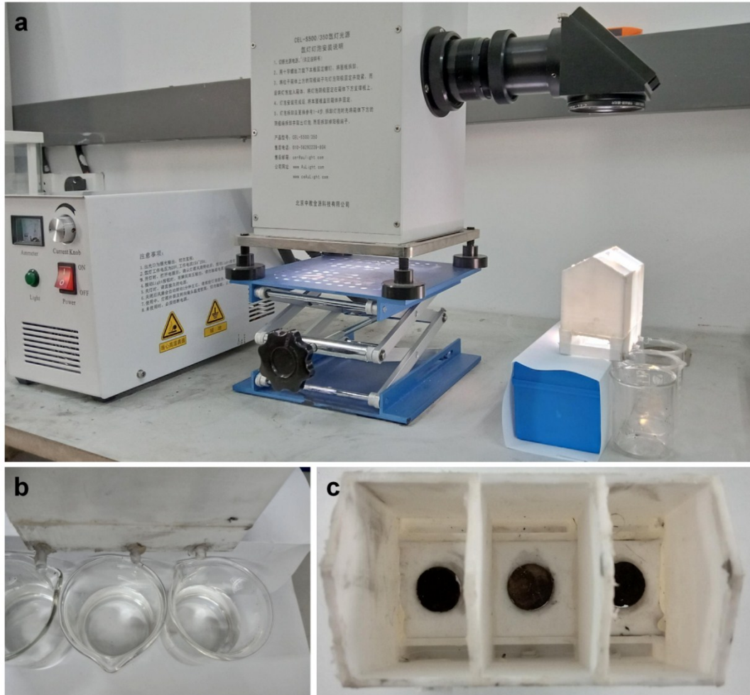
Figure S3. Evaporation experiment of corn stalk-based evaporators on solar simulator: (a) evaporation experiment, (b) freshwater collection, (c) evaporation chamber.
