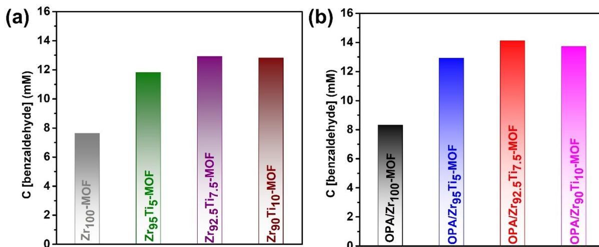
**Fig. S8.** Benzaldehyde concentration of (a) hydrophilic Zr<sub>100-x</sub>Ti<sub>x</sub>-MOF and (b) hydrophobic OPA/Zr<sub>100-x</sub>Ti<sub>x</sub>-MOF in two-phase system composed of benzyl alcohol (5.0 mL) and water (2.0 mL) catalyzed by 5.0 mg of photocatalysts under photoirradiation ( $\lambda > 420$  nm) after 3h reaction.
