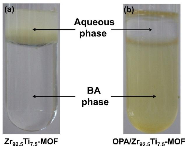
**Fig. S6.** The digital picture of two-phase system composed of BA/water containing (a) hydrophilic  $Zr_{92.5}Ti_{7.5}$ -MOF in aqueous phase and (b) hydrophobic OPA/ $Zr_{92.5}Ti_{7.5}$ -MOF in BA phase.
