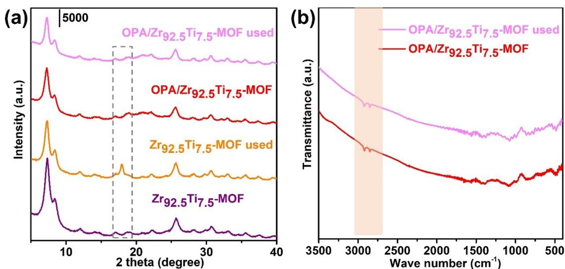
**Fig. S9.** (a) The XRD patterns and (b) FTIR spectra of Zr<sub>92.5</sub>Ti<sub>7.5</sub>-MOF and OPA/Zr<sub>92.5</sub>Ti<sub>7.5</sub>-MOF after recycling tests, compared with the samples before reaction.
