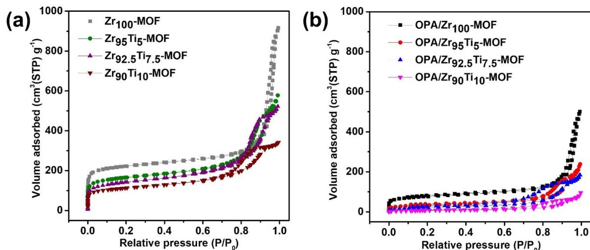
**Fig. S1** N<sub>2</sub> adsorption/desorption isotherms at 77 K of (a) Zr<sub>100-x</sub>Ti<sub>x</sub>-MOF and (b) OPA/Zr<sub>100-x</sub>Ti<sub>x</sub>-MOF.
