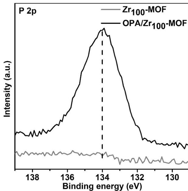
Fig. S2. XPS spectra of the synthesized samples: P 2p of Zr-MOF and OPA/Zr<sub>100</sub>-MOF.
