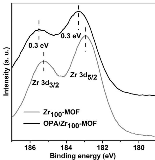
**Fig. S4.** The XPS spectra of the synthesized samples: Zr 3d of Zr<sub>100</sub>-MOF and OPA/Zr<sub>100</sub>-MOF.
