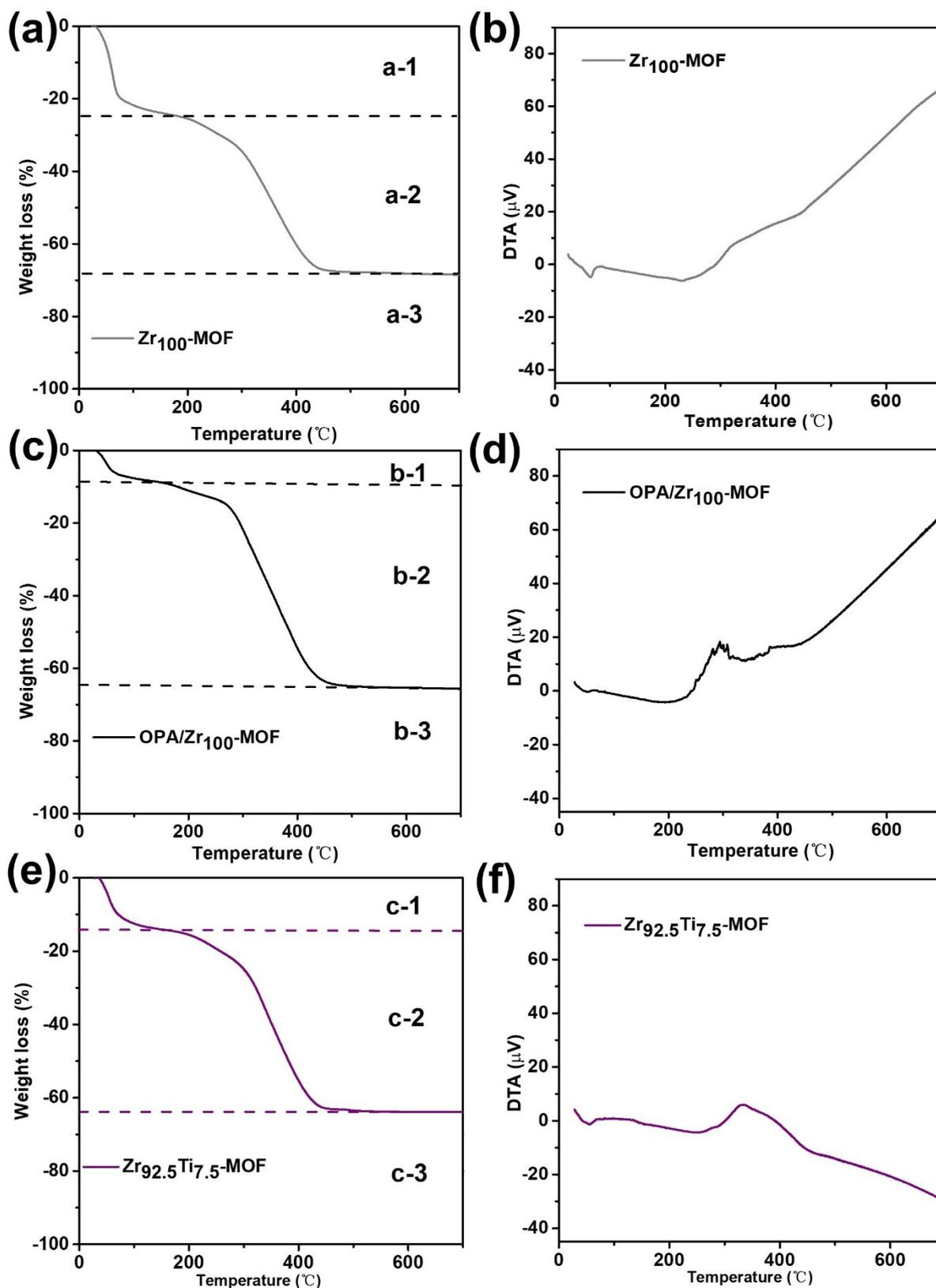
**Fig. S5.** (a, c, e, g) TG and (b, d, f, h) DTA profiles of  $Zr_{100}$ -MOF, OPA/ $Zr_{100}$ -MOF,  $Zr_{92.5}Ti_{7.5}$ -MOF and OPA/ $Zr_{92.5}Ti_{7.5}$ -MOF.
