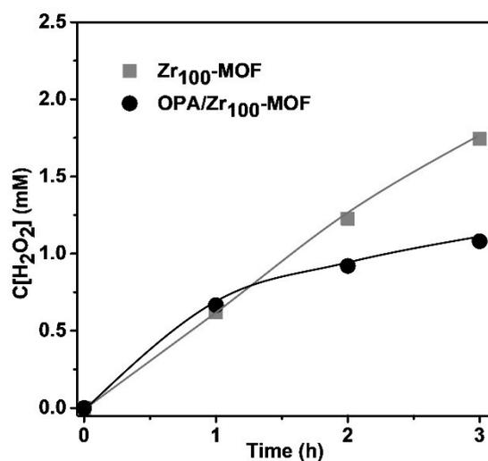
**Fig. S7.** H<sub>2</sub>O<sub>2</sub> production utilizing Zr<sub>100</sub>-MOF and OPA/ Zr<sub>100</sub>-MOF in single-phase system composed of an acetonitrile solution (5.0 mL) of BA (1.0 mL).
