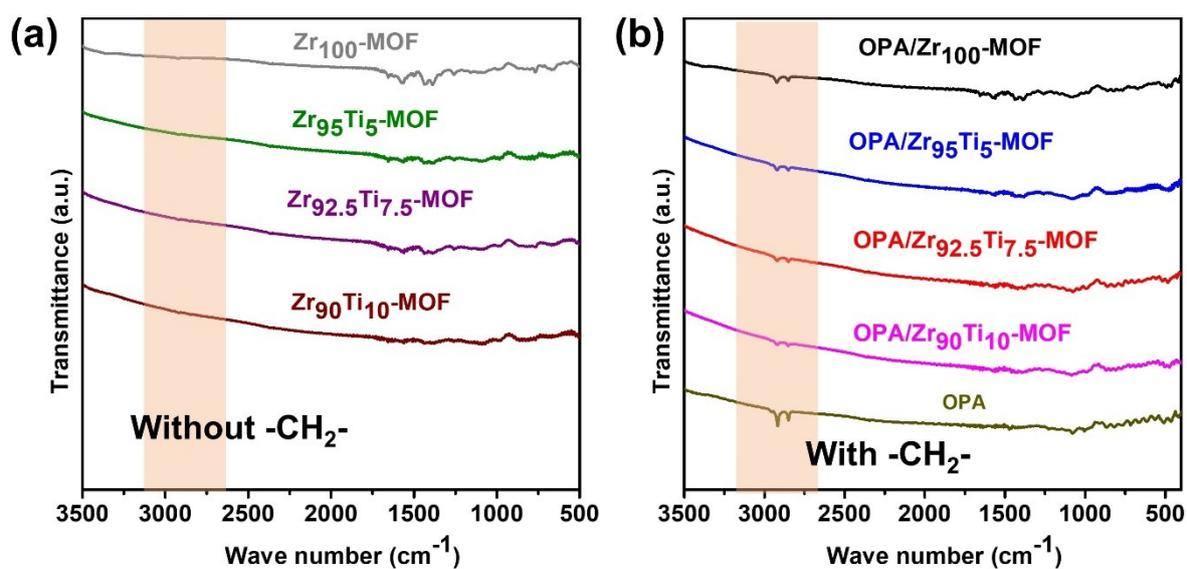
Fig. S3. FT-IR spectra of (a) Zr<sub>100-x</sub>Ti<sub>x</sub>-MOF and (b) OPA/Zr<sub>100-x</sub>Ti<sub>x</sub>-MOF.
