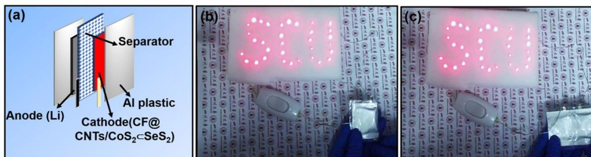
**Figure S10** (a) Schematic diagram of soft-packaged Li-SeS<sub>2</sub> battery; (b, c) Vivid photographs demonstration of the flexibility of the as-fabricated soft-packaged Li-SeS<sub>2</sub> battery based on the CF@CNTs/CoS<sub>2</sub>/SeS<sub>2</sub> cathode bending at 180° and after nearly 180°. The soft-packaged Li-SeS<sub>2</sub> battery can light up 33 red LEDs (nominal voltage of 2.0-2.2 V) in the flat and bent states.
