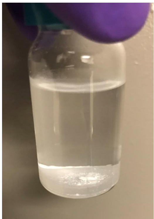
Fig S12. UiO-67 sunken to the bottom of a vial of water
