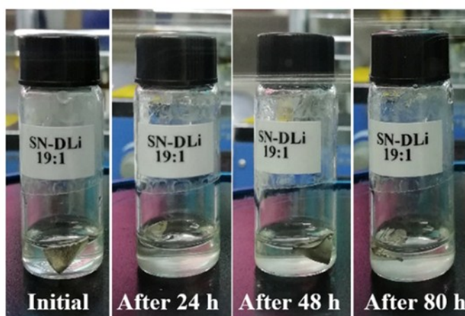
Fig. S5 Photographs of SN-DLi 19:1 electrolyte with Li-metal for different times at 60 °C.
