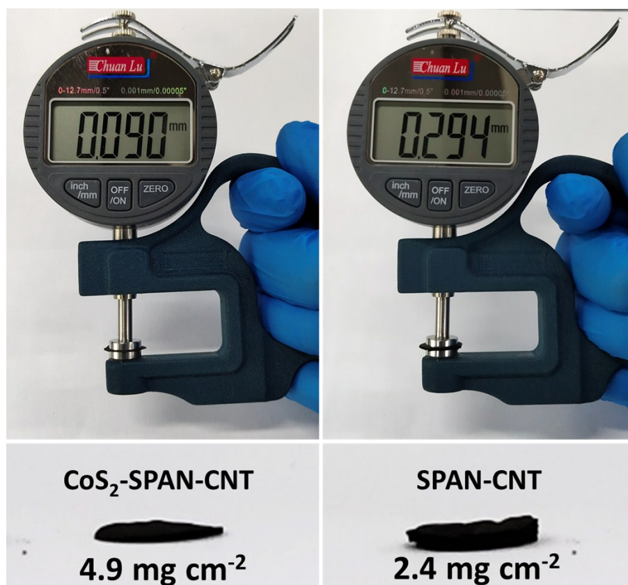
Fig. S4 The thickness comparison of CoS 2 -SPAN-CNT and SPAN-CNT at specific sulfur loadings.
