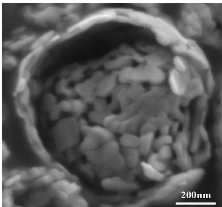
**Figure S2.** SEM image of broken microsphere.
