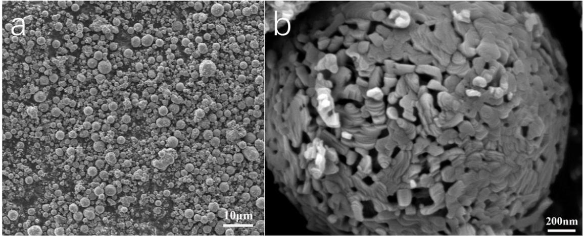
**Figure S1.** SEM images of V<sub>2</sub>O<sub>5</sub>-YS at a) low magnification and b) high magnification.
