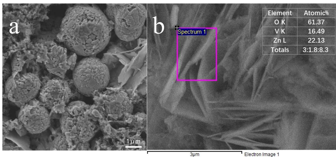
**Figure S9.** a) SEM image of  $V_2O_5$ -YS electrode soaked in aqueous electrolyte (nanoflakes:  $Zn_3V_2O_7(OH)_2 \cdot 2H_2O$ ) b) Element quantification of nanoflakes and the ratio of Zn, V, O is accorded with  $Zn_3V_2O_7(OH)_2 \cdot 2H_2O$ .
