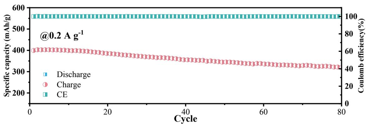
Figure S5. Cycling performance of the  $V_2O_5$ -YS cathode at current density of  $0.2 \text{ A g}^{-1}$ .
