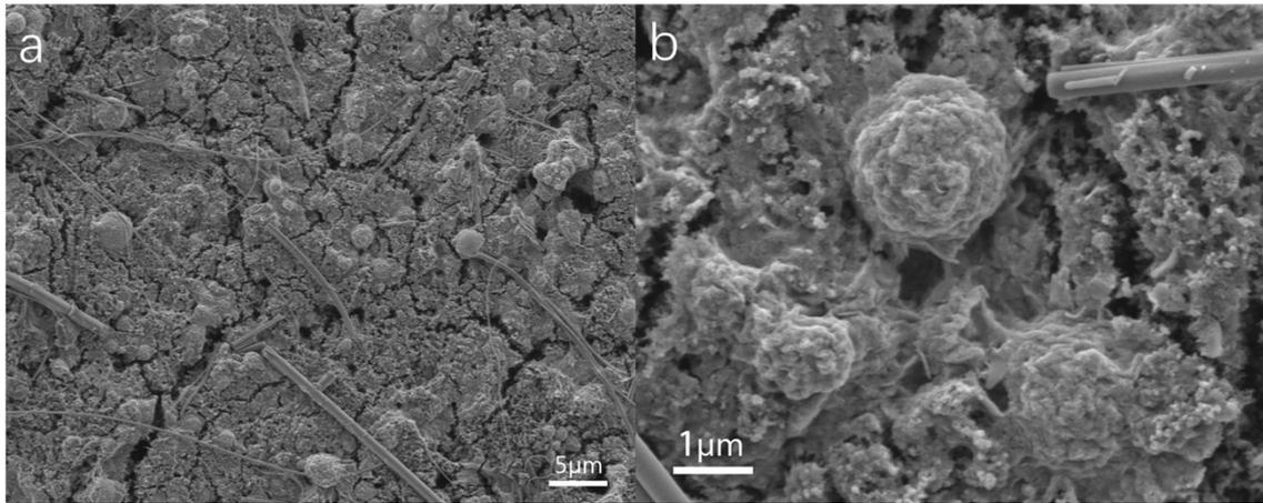
**Figure S4.** SEM Images of  $V_2O_5$ -YS cathode cycling for 100 cycles at the current density of  $1.0 \text{ A g}^{-1}$  at a) low magnification and b) high magnification, where nanofibers are fragments of glass fiber membrane.
