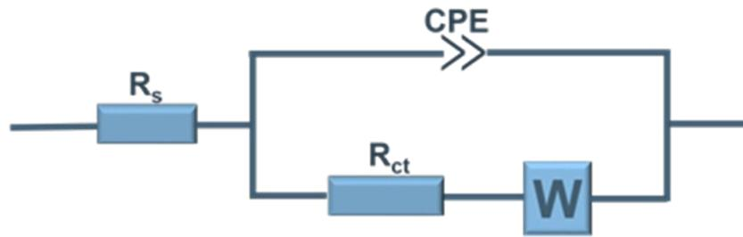
**Figure S7.** The equivalent circuit used for fitting the EIS curves of Figure 4c, where  $R_s$  = bulk resistance,  $R_{ct}$  = charge transfer resistance, CPE = constant phase element,  $W$ =Warburg impedance.
