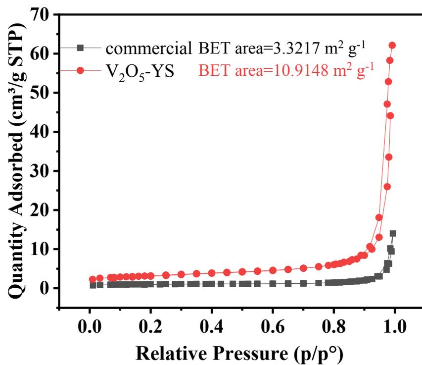
**Figure S3.** N<sub>2</sub> adsorption/desorption isotherms of commercial V<sub>2</sub>O<sub>5</sub> and as-prepared V<sub>2</sub>O<sub>5</sub>-YS at 77K.
