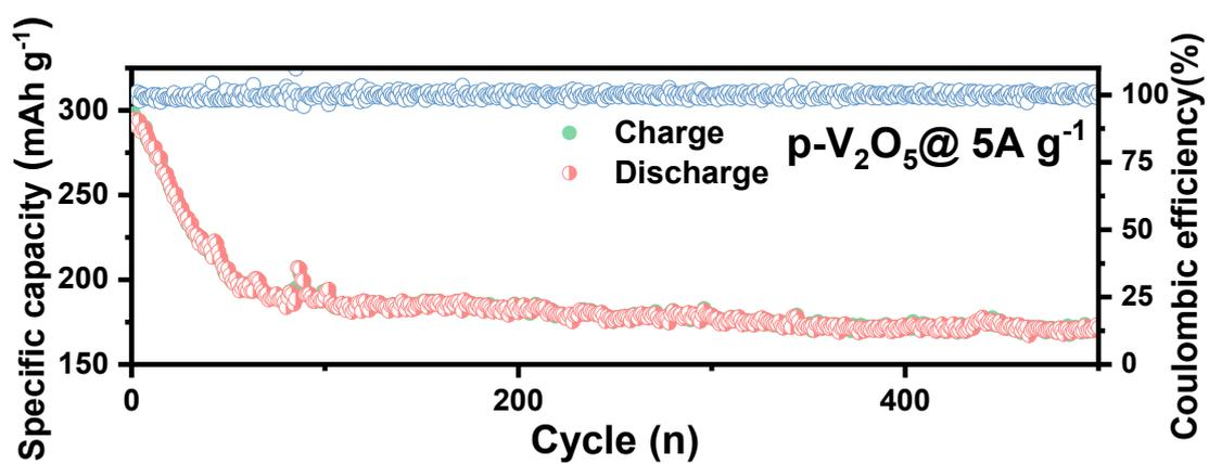
Figure S6. Cycling performance of the pristine  $V_2O_5$  at current density of  $5 \text{ A g}^{-1}$ .
