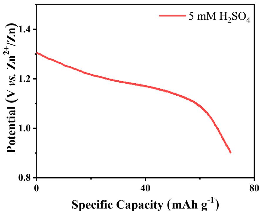
**Figure S8.** Galvanostatic discharge curve of the  $V_2O_5$ -YS cathode in a three-electrode cell in 5 mM  $H_2SO_4$  electrolyte.
