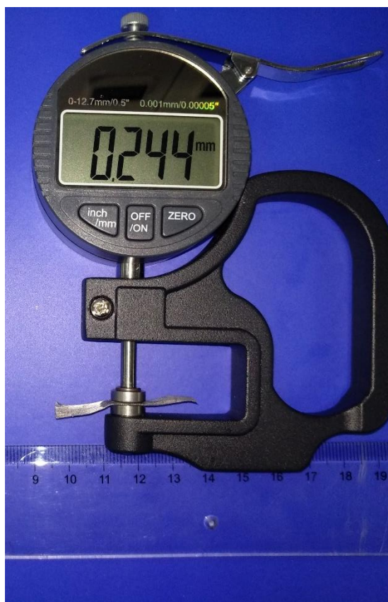
Figure S6. Photographs of a flexible supercapacitor based on N-MCN@GH film electrode and its compact configuration, with a thickness of 0.25 mm.
