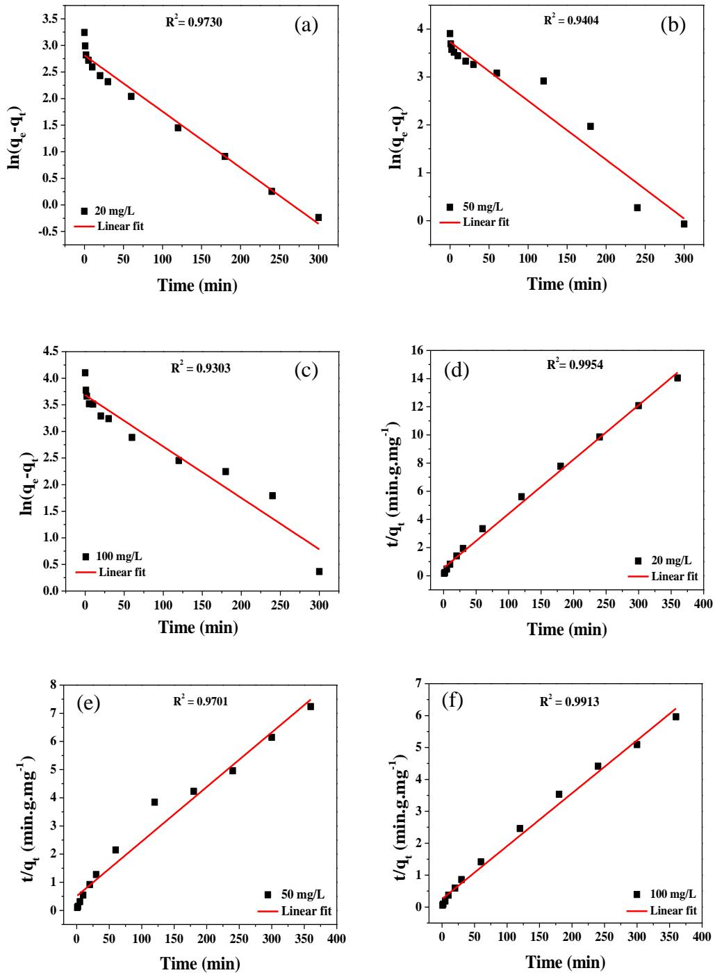
**Fig. S10** Fitted pseudo-first order kinetic rate model of MG 20 mg/L (a), MG 50 mg/L (b), MG 100 mg/L (c) and fitted pseudo-second order kinetic rate model of MG 20 mg/L (d), MG 50 mg/L (e), MG 100 mg/L (f) in the presence of ZIS-2.
