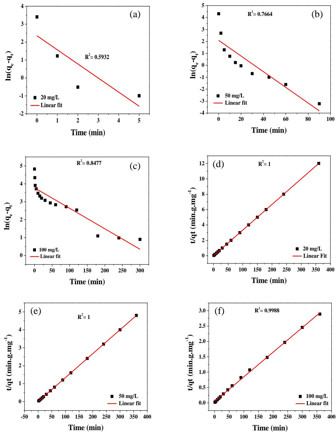
**Fig. S11** Fitted pseudo-first order kinetic rate model of MG 20 mg/L (a), MG 50 mg/L (b), MG 100 mg/L (c) and fitted pseudo-second order kinetic rate model of MG 20 mg/L (d), MG 50 mg/L (e), MG 100 mg/L (f) in the presence of ZIS-3.
