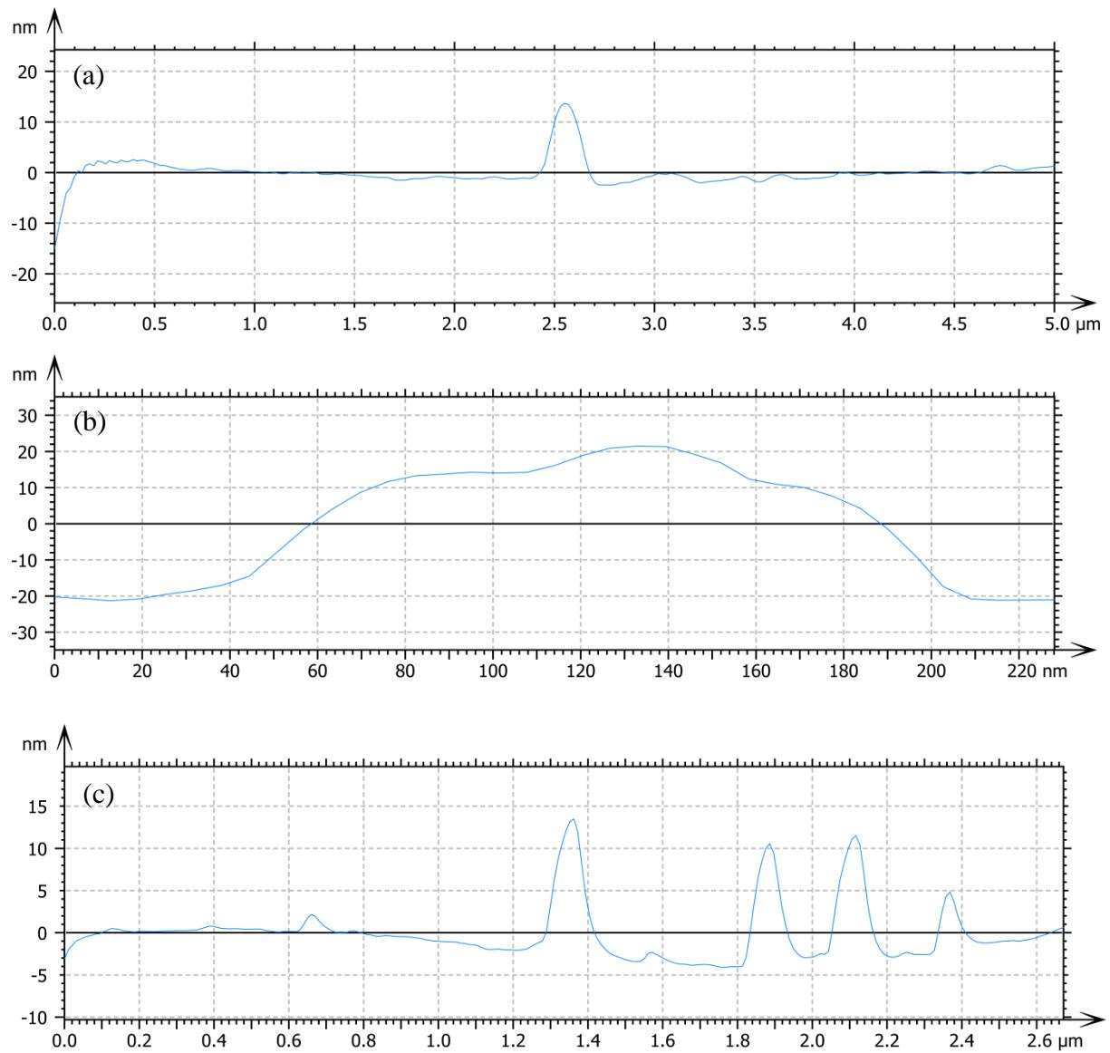
**Fig. S6** Thickness profile curve of the ZIS-1 (a), ZIS-2 (b) and ZIS-3 (c).
