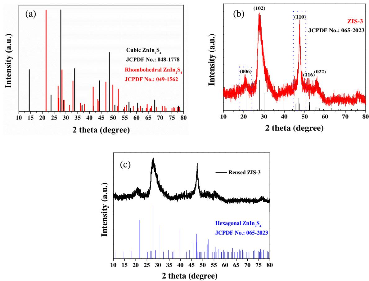
**Fig. S1** P-XRD pattern of standard cubic and rhombohedral  $\text{ZnIn}_2\text{S}_4$  (a), P-XRD of ZIS-3 with standard hexagonal  $\text{ZnIn}_2\text{S}_4$  (b) and reused ZIS-3 (c).
