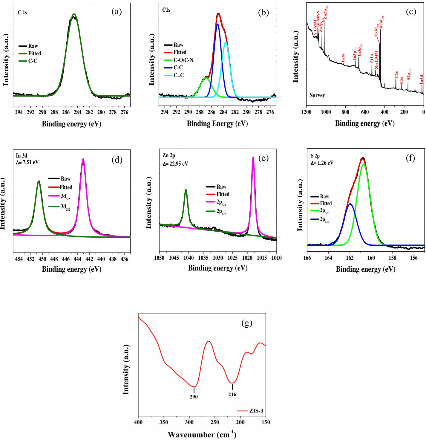
**Fig. S2** XPS spectra; C1s spectra of ZIS-1 (a), C1s spectra (b), survey spectra (c), core-level In3d spectra (d), core-level Zn 2p spectra (e), core-level S2p spectra (f), of reused ZIS-3 and far-IR spectra of ZIS-3 (g).
