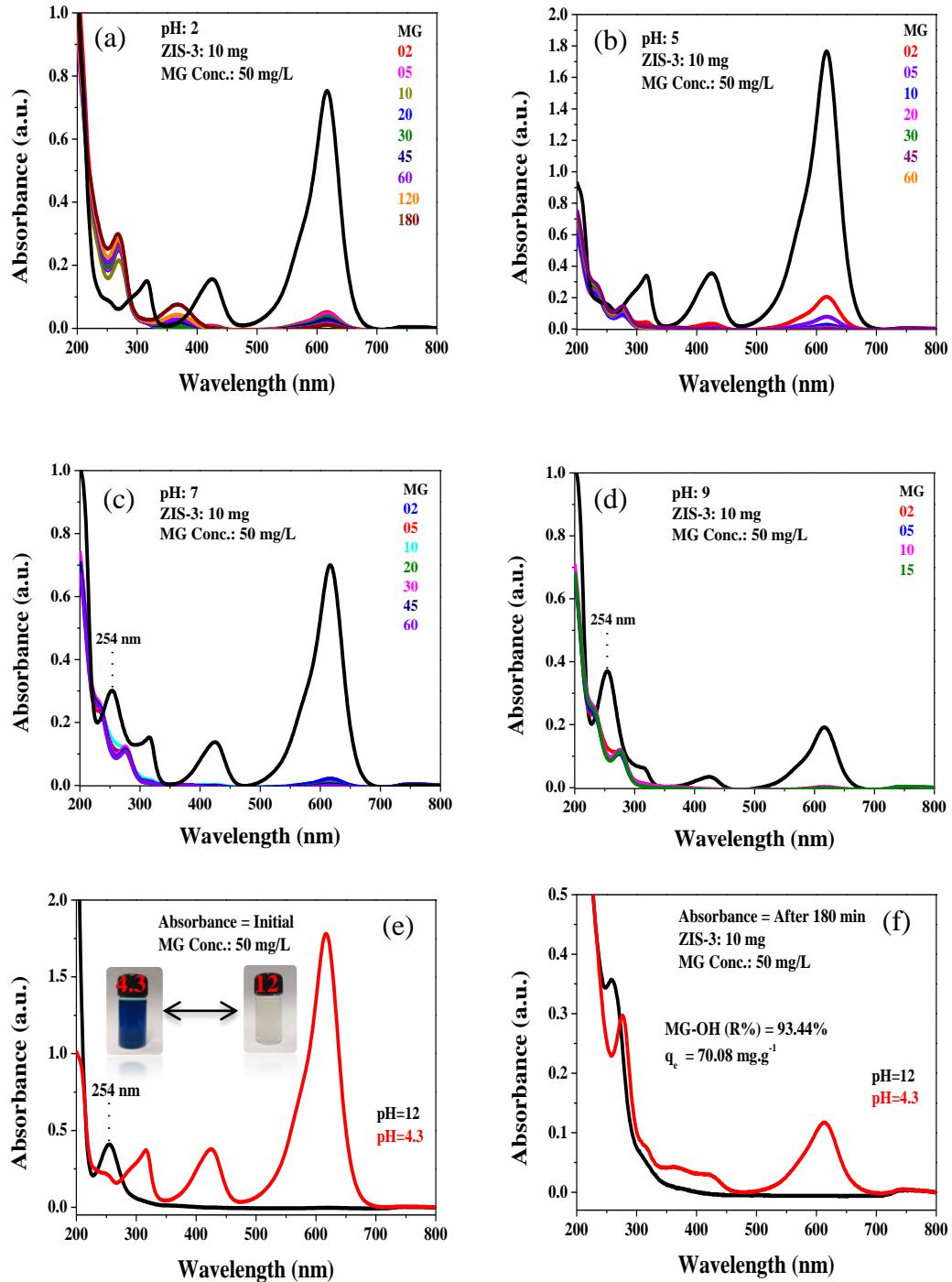
**Fig. S19** UV-Vis spectra of MG (50 mg/L) adsorption at pH 2 (a), pH 5 (b), pH 7 (c), pH 9 (d) and initial absorbance of MG at pH 12 and pH 4.3 (e) after adsorption at pH 12 (f) using ZIS-3.
