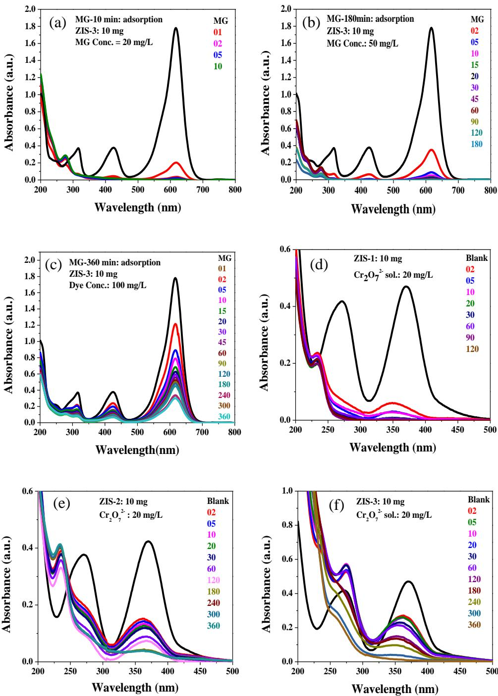
**Fig. S15** UV-Vis spectra of adsorption of MG at 20 mg/L (a), 50 mg/L (b), 100 mg/L (c) using ZIS-3 and Cr<sub>2</sub>O<sub>7</sub><sup>2-</sup> adsorption using ZIS-1 (d), ZIS-2 (e) and ZIS-3 (f) at 20 mg/L solution.
