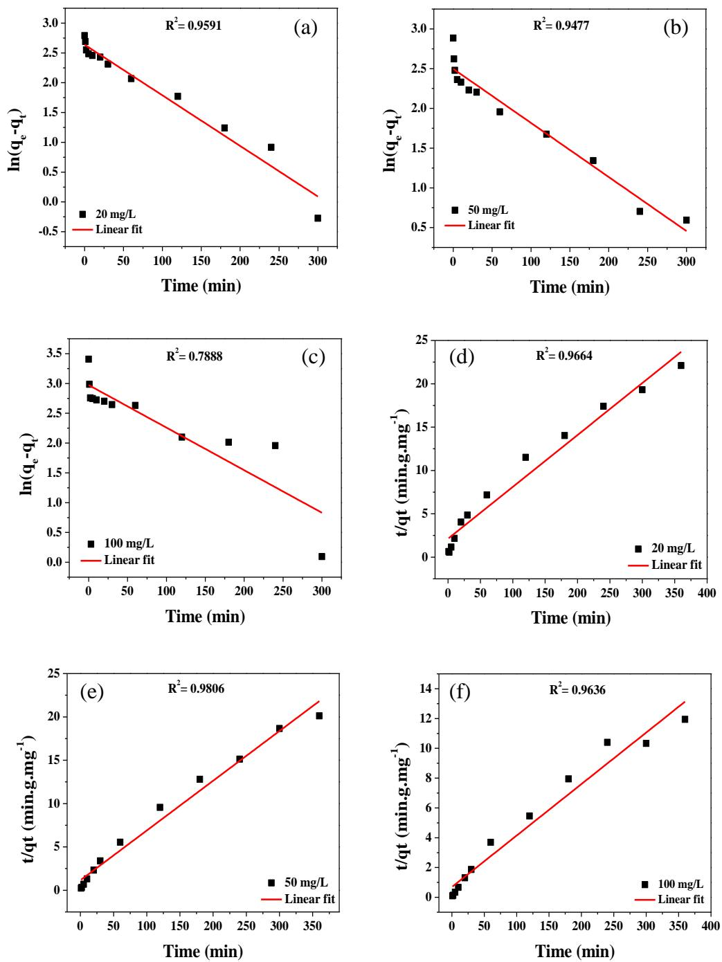
**Fig. S9** Fitted pseudo-first order kinetic rate model of MG 20 mg/L (a), MG 50 mg/L (b), MG 100 mg/L (c) and fitted pseudo-second order kinetic rate model of MG 20 mg/L (d), MG 50 mg/L (e), MG 100 mg/L (f) in the presence of ZIS-1.
