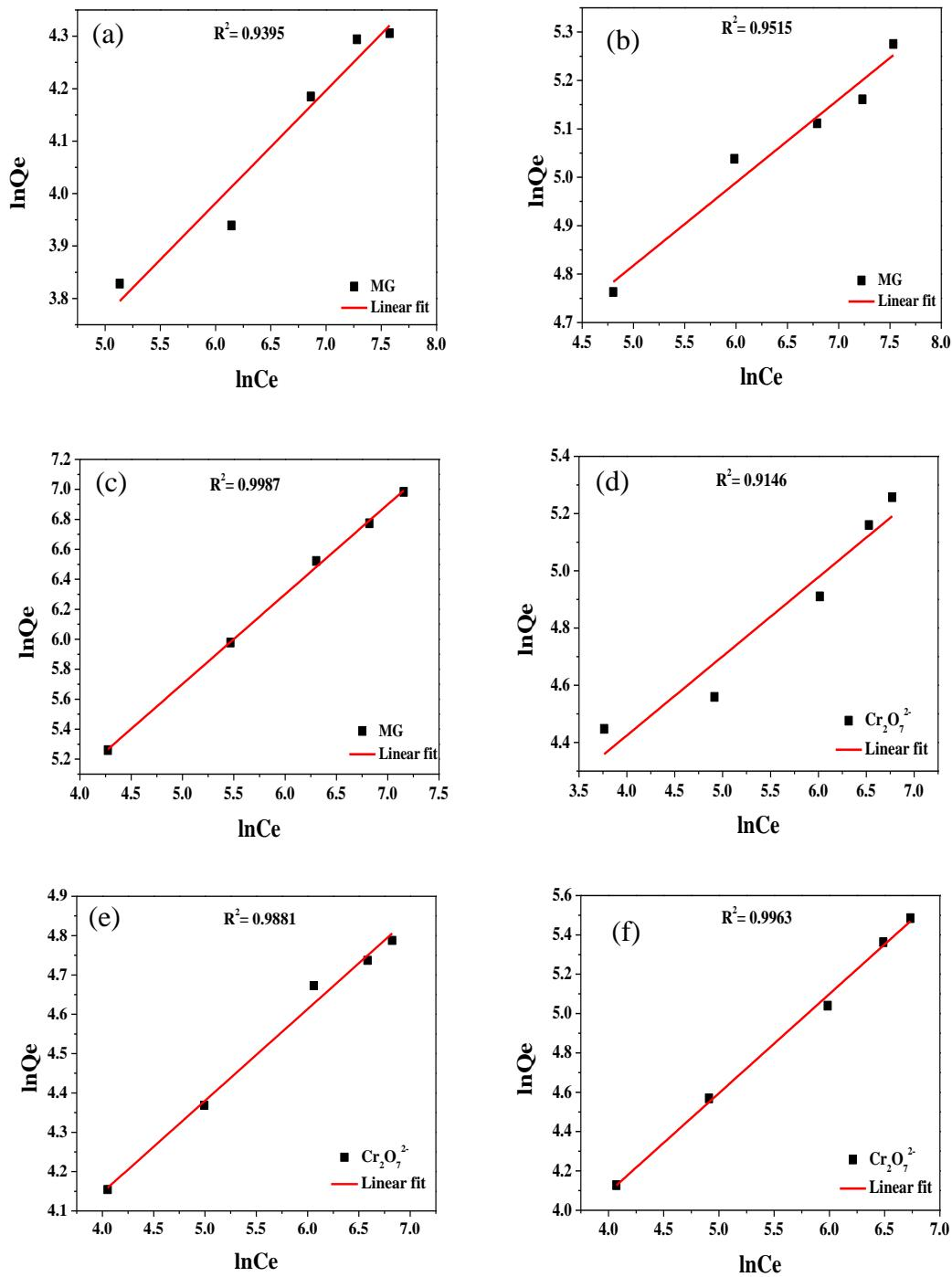
**Fig. S8** Fitted Freundlich adsorption isotherm model of ZIS-1 (a), ZIS-2 (b), ZIS-3 (c) for the MG adsorption and ZIS-1 (d), ZIS-2 (e), ZIS-3 (f) for the adsorption of  $\text{Cr}_2\text{O}_7^{2-}$ .
