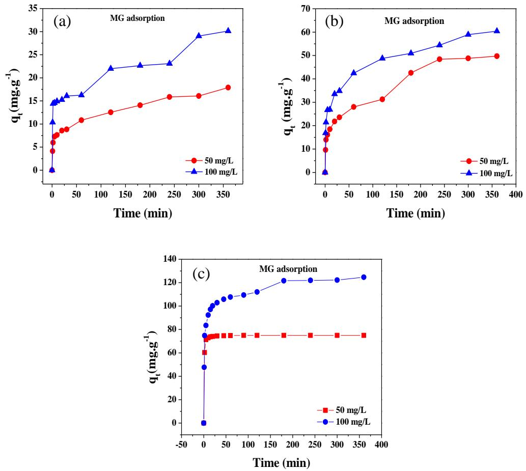
**Fig. S13** Effect of contact time on the adsorption of MG using ZIS-1 (a), ZIS-2 (b), and ZIS-3 (c) at the solution concentration of 50  $\text{mg}\cdot\text{L}^{-1}$  and 100  $\text{mg}\cdot\text{L}^{-1}$ .
