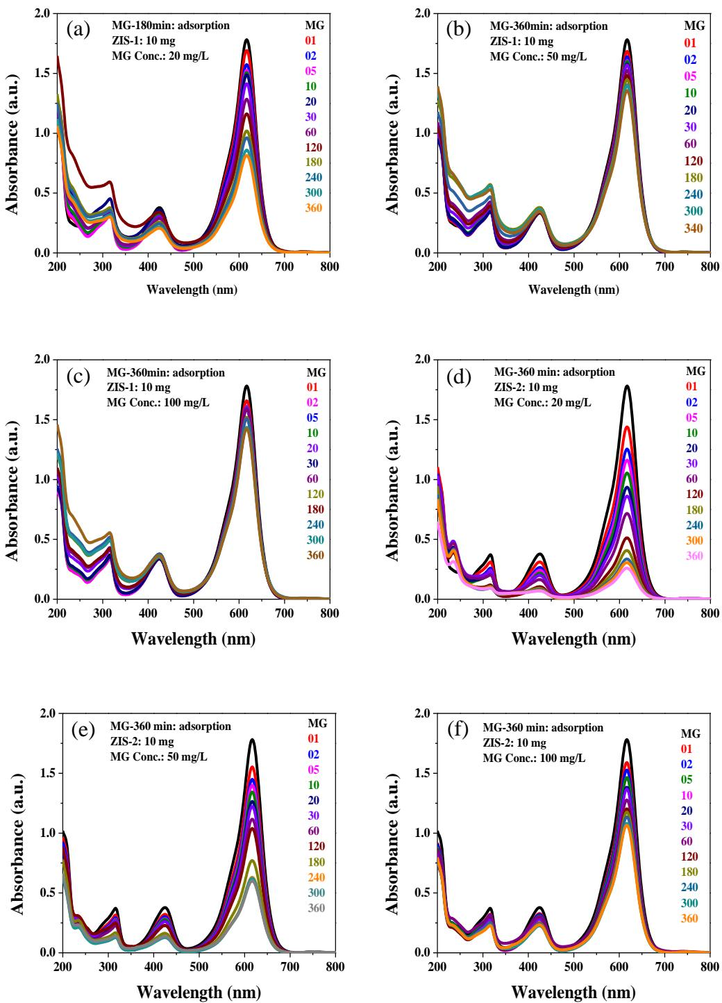
**Fig. S14** UV-Vis spectra of adsorption of MG at 20 mg/L (a), 50 mg/L (b), 100 mg/L (c) using ZIS-1 and MG adsorption at 20 mg/L (d), 50 mg/L (e), 100 mg/L (f) using ZIS-2.
