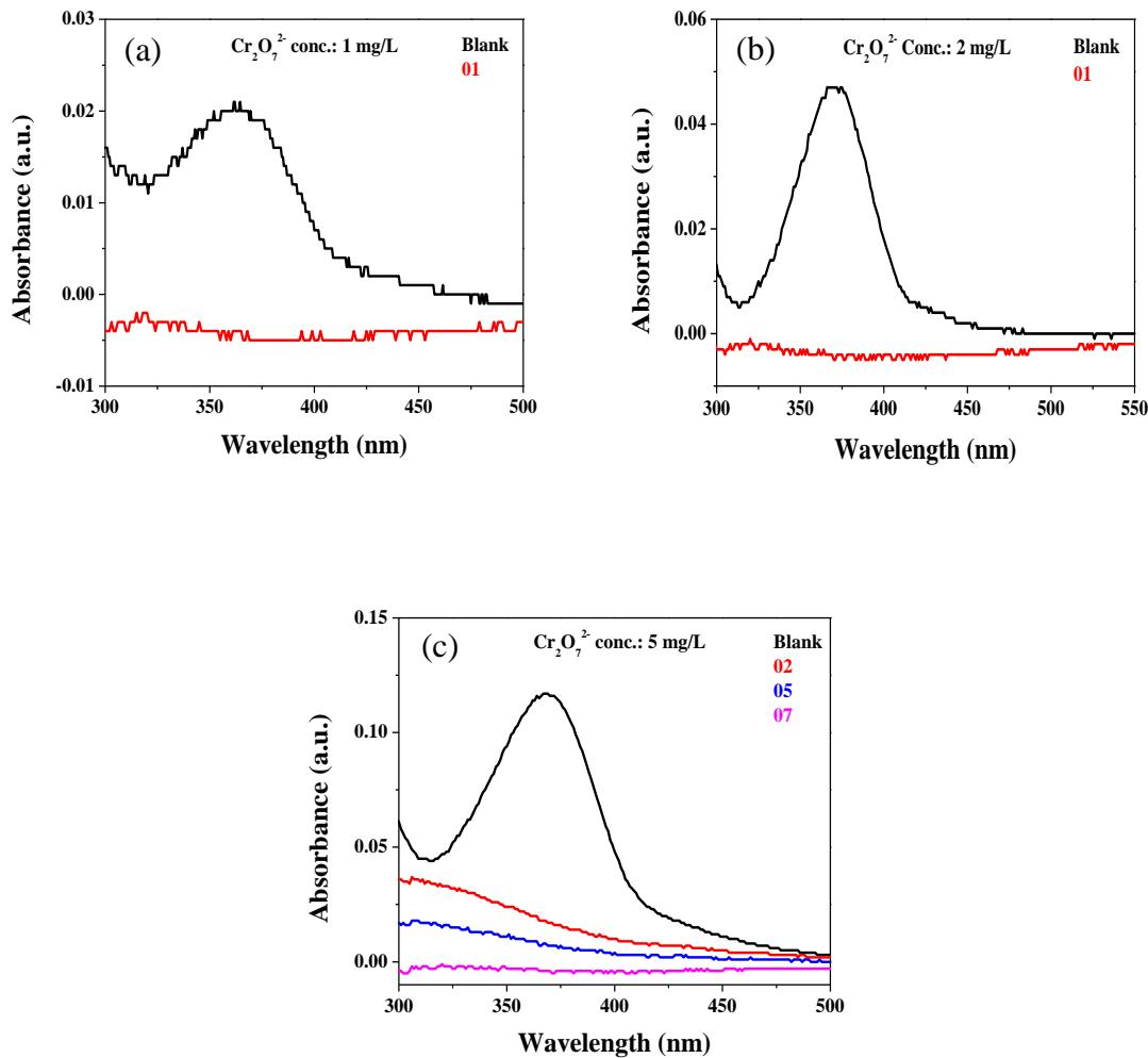
**Fig. S18** UV-Vis spectra of adsorption of Cr<sub>2</sub>O<sub>7</sub><sup>2-</sup> at 1 mg/L (a), 2 mg/L (b) and 5 mg/L of solution concentration using ZIS-1.
