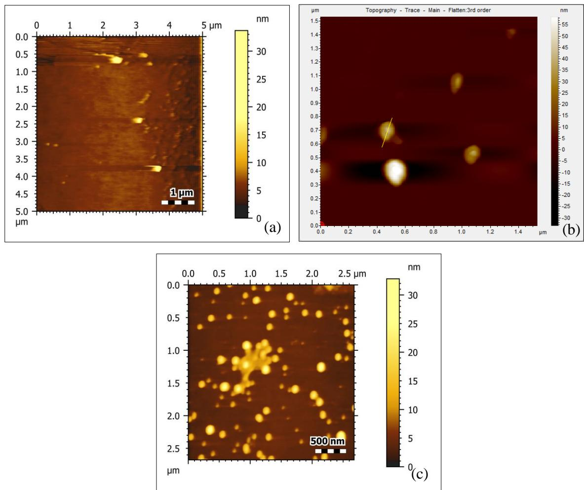
**Fig. S5** AFM topography of the ZIS-1 (a), ZIS-2 (b) and ZIS-3 (c).
