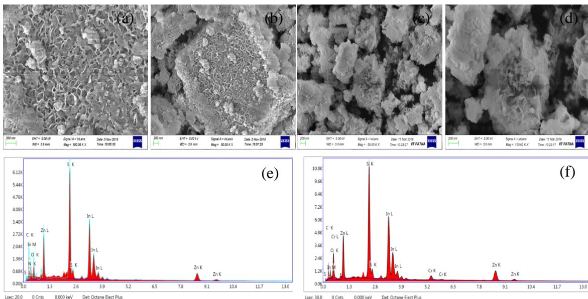
**Fig. S21** FE-SEM micrograph of ZIS-3: (a-b) after MG adsorption, (c-d) after  $\text{Cr}_2\text{O}_7^{2-}$  adsorption; EDS line mapping of ZIS-3: (e) after MG adsorption, (f) after  $\text{Cr}_2\text{O}_7^{2-}$  adsorption.
