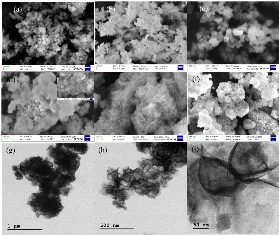
**Fig. S3** FE-SEM micrograph: SE2 mode at 100K magnification (a), InLens mode at 100K magnification (b), InLens mode at 200K magnification (c) of ZIS-1; InLens mode at 100K inset with SE2 mode at 200K magnification (d) of ZIS-2; SE2 mode at 100K magnification (e), InLens mode at 50.52K magnification (f) of ZIS-3; TEM micrograph of ZIS-3 (g-i).
