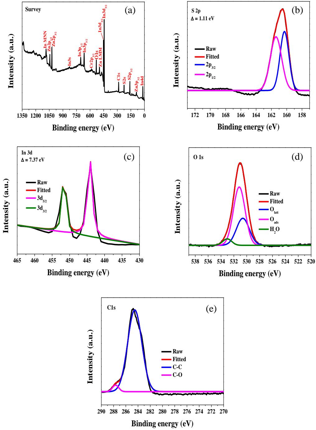
**Fig. S22** XPS spectra of ZIS-3 after  $\text{Cr}_2\text{O}_7^{2-}$  adsorption; survey spectra (a), core-level S 2p spectra (b), core-level In3d spectra (c), core-level O1s spectra (d) and core-level C 1s spectra (e).
