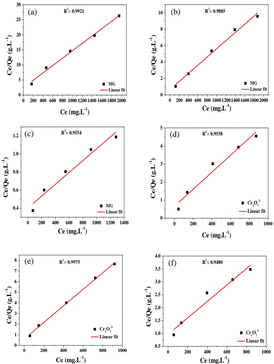
**Fig. S7** Fitted Langmuir adsorption isotherm model of ZIS-1 (a), ZIS-2 (b), ZIS-3 (c) for MG adsorption and ZIS-1 (d), ZIS-2 (e), ZIS-3 (f) for the adsorption of  $\text{Cr}_2\text{O}_7^{2-}$ .
