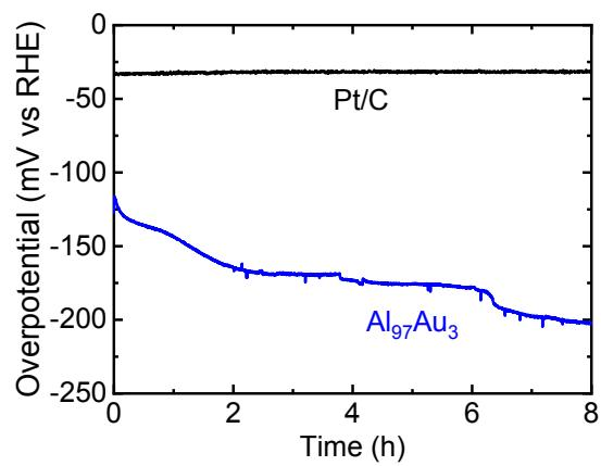
Figure S2. The reaction stability of Al<sub>97</sub>Au<sub>3</sub> electrode in 0.5 M H<sub>2</sub>SO<sub>4</sub> at a constant hydrogen evolution current of 10 mA cm<sup>-2</sup>.
