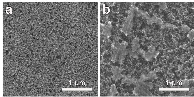
Figure S3. Comparison of the nanoporous microstructure (SEM images) for (a) the  $\text{Al}_{80}\text{Ni}_6\text{Co}_3\text{Mn}_3\text{Y}_5\text{Au}_3$  electrode and (b)  $\text{Al}_{87}\text{Au}_3$  electrode after 2 hours reaction in 0.5 M  $\text{H}_2\text{SO}_4$  at 200 mV (versus 3.5 M  $\text{Ag}/\text{AgCl}$ ). The ligaments coarsen and the nanopores get closed for the  $\text{Al}_{87}\text{Au}_3$  electrode.
