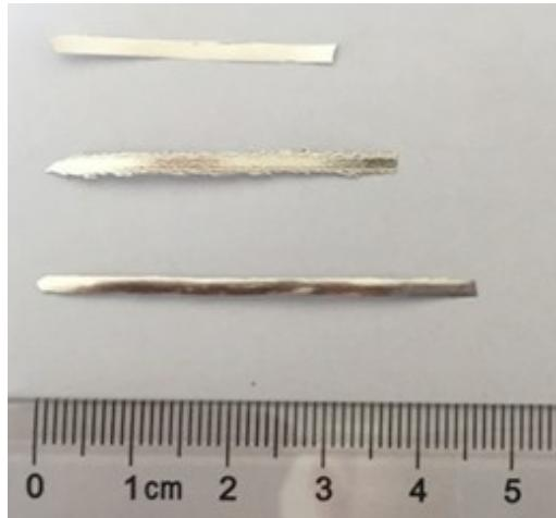
Figure S1. The optical image of ribbons for  $\text{Al}_{97}\text{Au}_3$ ,  $\text{Al}_{85}\text{Ni}_7\text{Y}_8$  and  $\text{Al}_{80}\text{Ni}_6\text{Co}_3\text{Mn}_3\text{Y}_5\text{Au}_3$ . The thickness of the electrode is 20  $\mu\text{m}$ , the width of the electrode is about 1.8 mm, the length of the electrode for electrochemical measurement is about 1cm.
