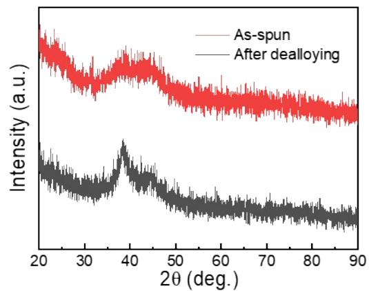
Figure S4. XRD patterns of as-spun and dealloyed  $\text{Al}_{80}\text{Ni}_6\text{Co}_3\text{Mn}_3\text{Y}_5\text{Au}_3$ .
