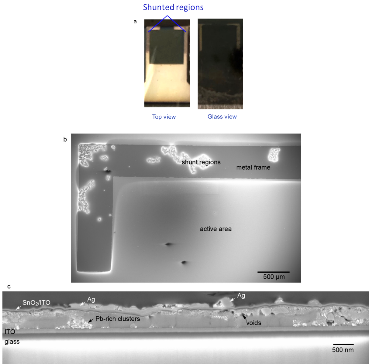
Figure S4: a) semitransparent solar cell reverse biased from 0 V to -5 V in 3 min steps of -0.1 V showing visible burn marks. The top Ag contact can be seen from the glass side. b-c) Top view and focused ion beam-prepared cross-section scanning electron microscopy images of shunted areas.
