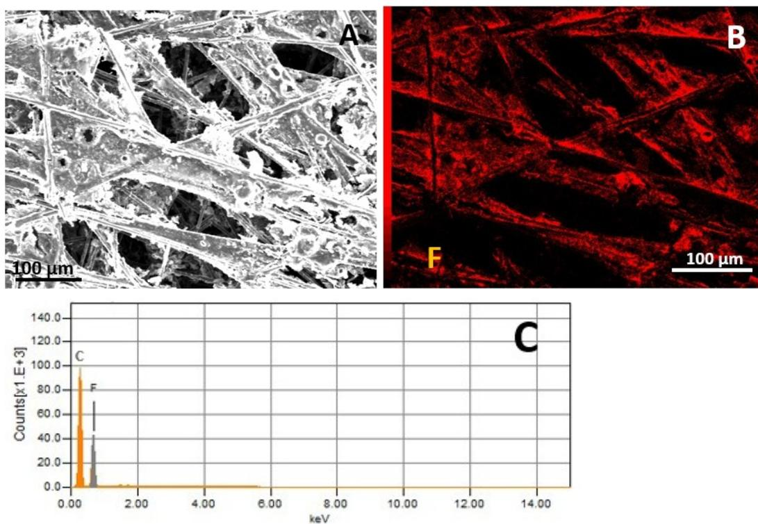
Figure S5. SEM image (a), EDS map (b), and EDS spectrum (c) of bare carbon paper. The data show that the electrode contains carbon and fluorine. The fluorine comes from PTFE used to treat the carbon paper.
