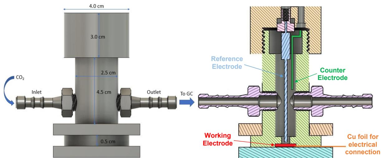
Figure S1. Schematics of custom-made cell for gas collection. The reference and counter electrodes were positioned through o-ring sealed ports on the top of the cell. The working electrode was placed on the bottom of the cell and was hermetically sealed using a compressed o-ring. The figure on the right highlights the positions of the three electrodes.
