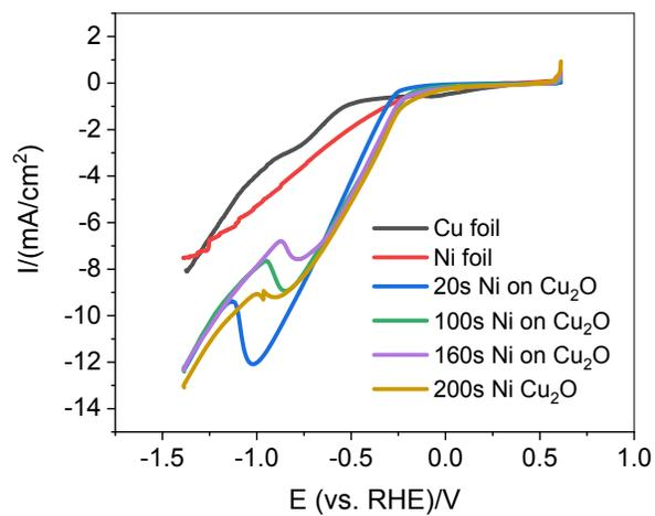
Figure S3. Linear sweep voltammogram (LSV) of bare carbon, Cu foil, Ni foil, and Cu<sub>2</sub>O thin films with 20 s, 100 s, 160 s, and 200 s of electrodeposited Ni.
