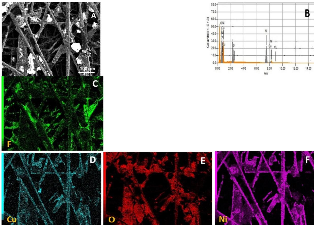
Figure S6. SEM image (a), spectrum (b), and elemental mapping (c-f) of a  $\text{Cu}_2\text{O}$  on carbon paper electrode modified with 500 s of Ni electrodeposition.
