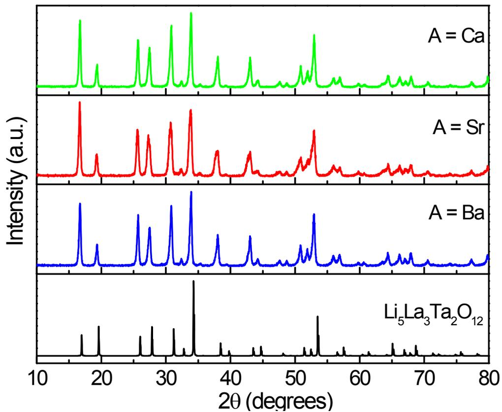
**Fig. S1.** XRD patterns of garnet-type  $\text{Li}_{6.5}\text{La}_{2.9}\text{A}_{0.1}\text{Zr}_{1.4}\text{Ta}_{0.6}\text{O}_{12}$  (A = Ca, Sr, Ba) pellets prepared by SPS process and the calculated pattern of cubic garnet-type  $\text{Li}_5\text{La}_3\text{Ta}_2\text{O}_{12}$  (space group:  $Ia\bar{3}d$ ;  $a = 12.80 \text{ \AA}$ ) using the PowderCell program.<sup>3</sup>
