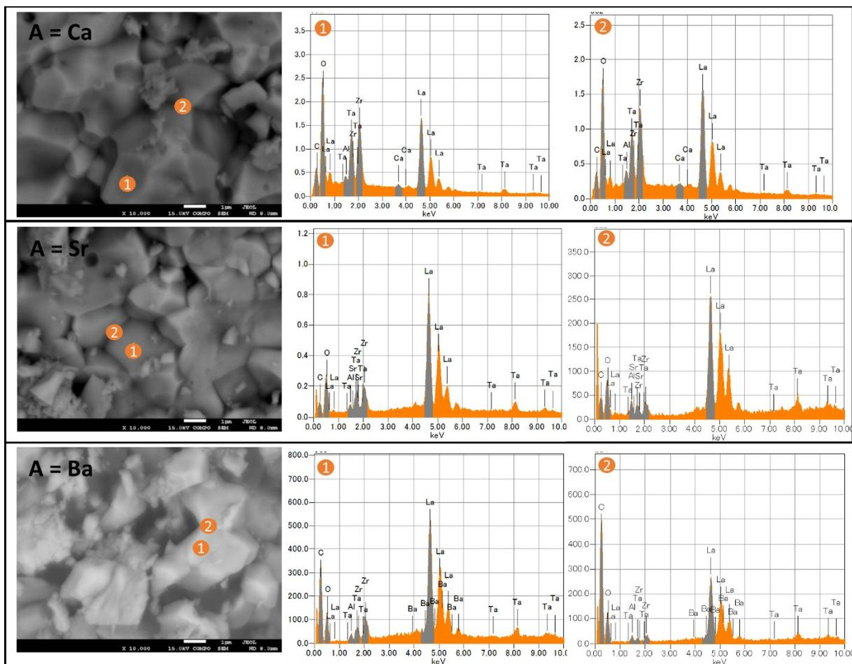
**Fig. S3.** SEM images and corresponding EDS spectra ((grain (1) and grain-boundary (2)) of  $\text{Li}_{6.5}\text{La}_{2.9}\text{A}_{0.1}\text{Zr}_{1.4}\text{Ta}_{0.6}\text{O}_{12}$  (A = Ca, Sr, Ba) garnet electrolytes prepared by spark plasma sintering technique.
