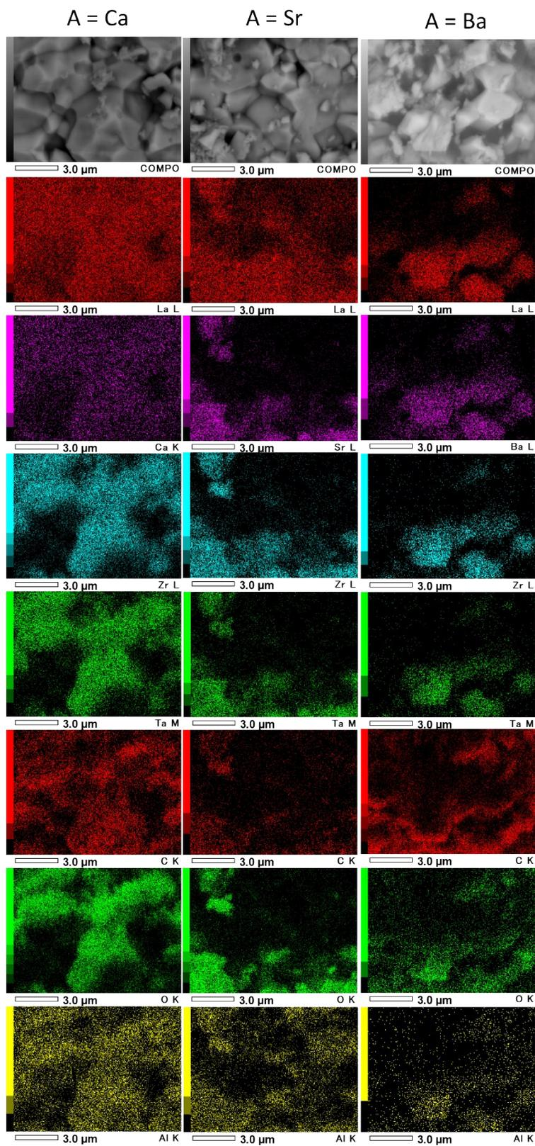
**Fig. S2.** SEM images and corresponding elemental mapping of  $\text{Li}_{6.5}\text{La}_{2.9}\text{A}_{0.1}\text{Zr}_{1.4}\text{Ta}_{0.6}\text{O}_{12}$  (A = Ca, Sr, Ba) garnet electrolytes prepared by spark plasma sintering technique.
