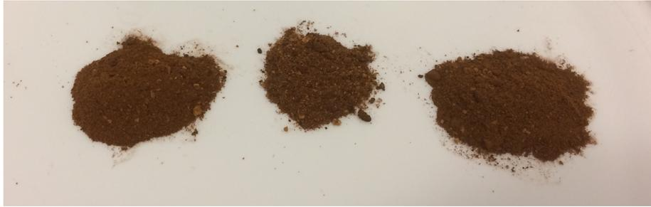
**Figure S4.** Photograph of HCP1 (left), HCP1, Ca(OH)<sub>2</sub> treated (centre) and HHCP2, NaOH-treated (right).
