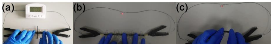
Figure S14. (a) Photographs of electrical clock powered by two devices in series in compressing state. Photographs of LED lamp powered by three devices in series in compressing state (b) and bending state (c).
