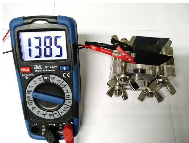
Figure S20. Photograph of the Zn-air battery employing the commercial cathode, giving an open-circuit potential of 1.385 V.
