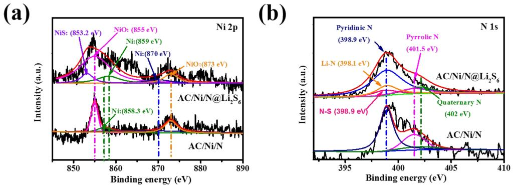
**Fig. S11** (a) High-resolution XPS spectra for Ni 2p and (b) N 1s before and after cycling.
