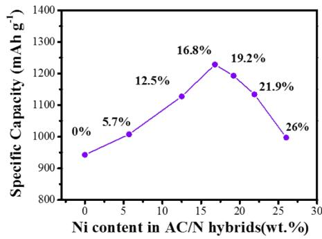
**Fig. S6.** Capacity optimization of Ni content in the AC/Ni/N hybrids.
