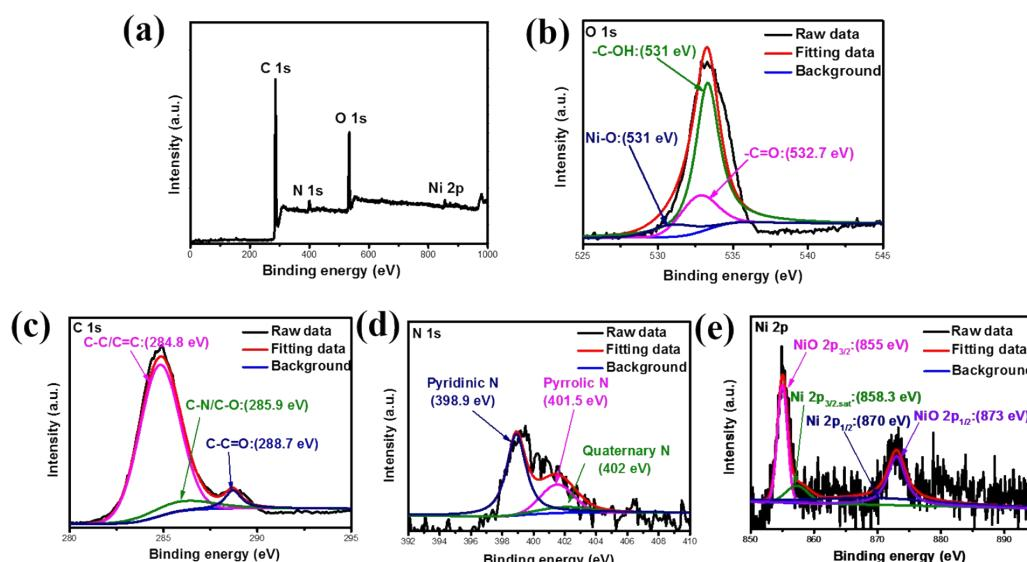
**Fig. S2.** (a) XPS analysis of AC/Ni/N composites and high-resolution spectrum of (b)O 1s; (c)C 1s; (d)N 1s; and (e)Ni 2p; respectively.
