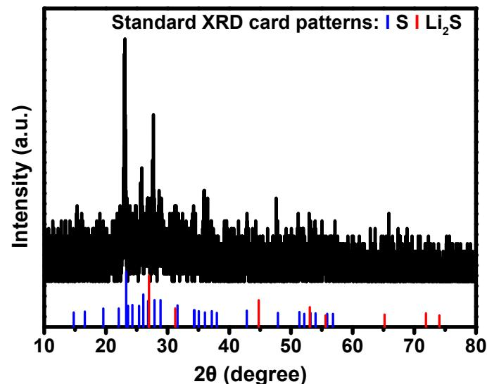
**Fig. S10.** XRD patterns of AC/Ni/N coated separator after cycling and standard XRD patterns sulfur and Li<sub>2</sub>S powder.
