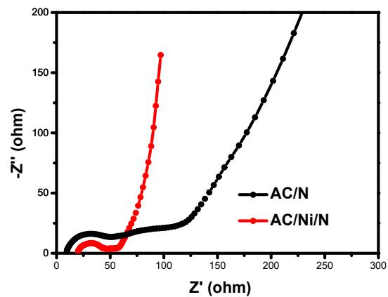
**Fig. S8.** Nyquist plots of cells with AC/N and AC/Ni/N modified separator after cycling at 1.5C.
