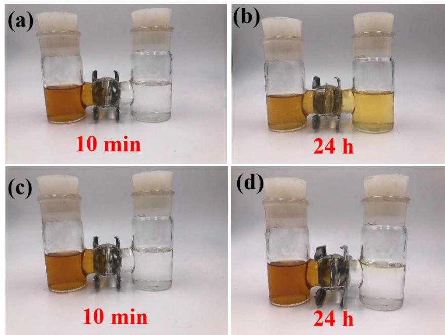
**Fig. S9.** Permeation experiments with an H-type permeation device with (a, b) a pristine separator; and (c, d) an AC/Ni/N coated separator after 24 h.
