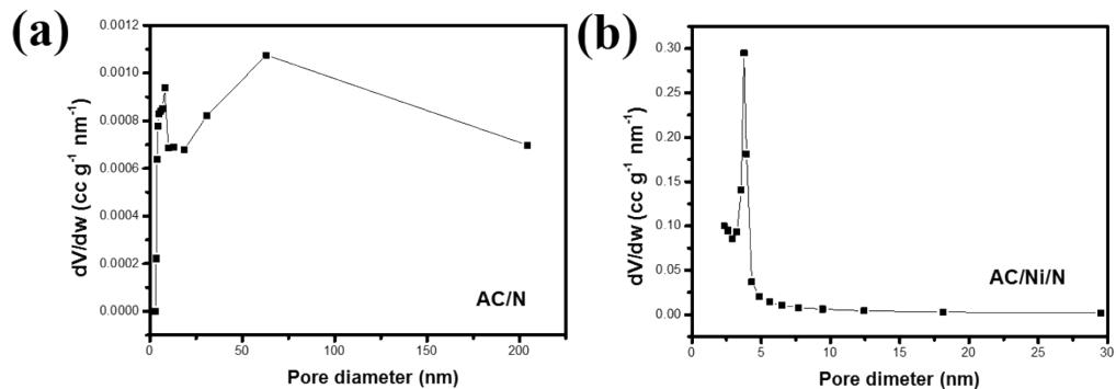
**Fig. S3.** The pore size distributions of AC/N and AC/Ni/N hybrids.
