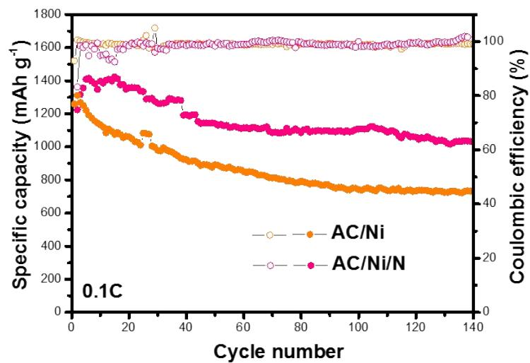
**Fig. S7.** The cycle performance of the cell of AC/Ni and AC/Ni/N modified separator.
