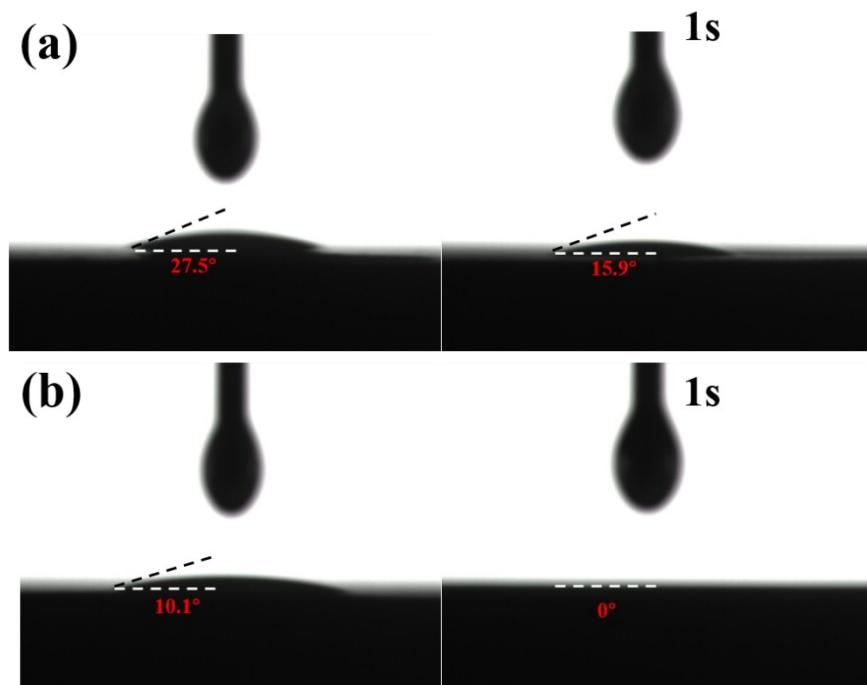
**Fig. S5.** Contact angle measurements of (a) pristine separator; and (b) AC/Ni/N coated separator for the electrolyte.
