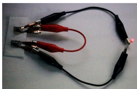
Fig. S7. Optical image of an LED lighted by two EMSC with gelatin sheet substrate connected in series under a current density of 0.1 \text{ mA cm}^{-2} .
