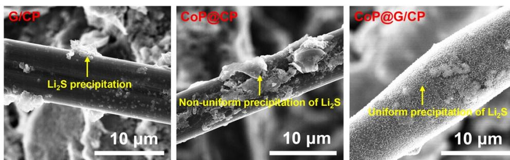
Fig. S14. SEM observations of  $\text{Li}_2\text{S}$  nucleation on the surface of G/CP, CoP@CP and CoP@G/CP, respectively.
