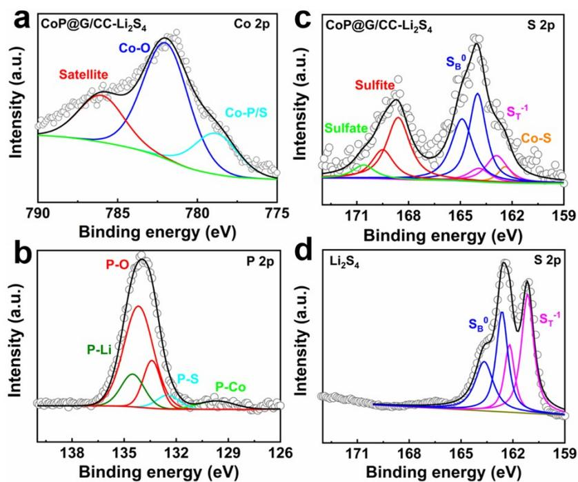
**Fig. S7.** XPS spectra of (a) Co 2p of CoP@G/CC after interacting with Li<sub>2</sub>S<sub>4</sub>, (b) P 2p of CoP@G/CC after interacting with Li<sub>2</sub>S<sub>4</sub>, (c) S 2p of CoP@G/CC after interacting with Li<sub>2</sub>S<sub>4</sub> and (d) S 2p of bare Li<sub>2</sub>S<sub>4</sub>.
