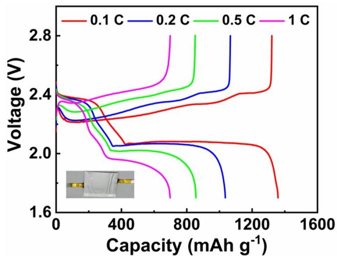
**Fig. S20.** Galvanostatic charge/discharge profiles of assembled pouch cell with CoP@G/CC-S cathode at different current densities.
