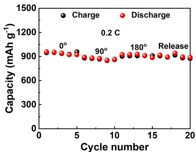
**Fig. S21.** Cycling performance of the pouch cell under bent-release states.
