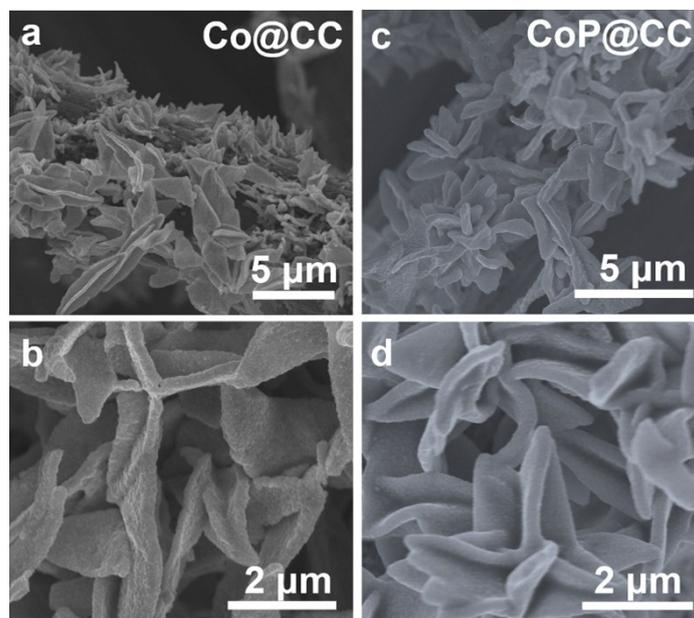
**Fig. S3.** SEM images of (a, b) Co@CC and (c, d) CoP@CC.
