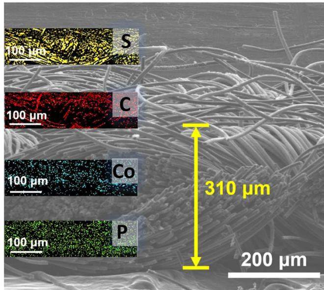
**Fig. S19.** Cross-sectional SEM/EDS characterization of the CoP@G/CC-S cathode with a sulfur loading of  $10.83 \text{ mg cm}^{-2}$ .
