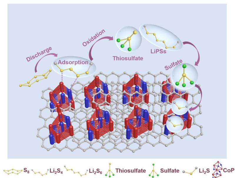
Fig. S16. Schematic illustration of  $S_8$  evolution on CoP@G/CC hybrid host.
