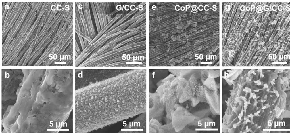
**Fig. S17.** SEM images of CC-S (a, b), G/CC-S (c, d), CoP@CC-S (e, f) and CoP@G/CC-S (g, h) cathodes before (a, c, e, g) and after (b, d, f, h) 100 cycles.
