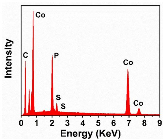
Fig. S10. EDS spectrum of CoP@G/CC-S cathode with a sulfur mass loading of 2.31 mg cm<sup>-2</sup>.
