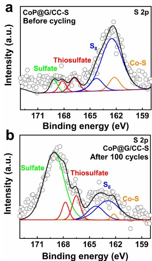
Fig. S15. XPS S 2p analysis of CoP@G/CC-S cathode before and after 100 cycles.
