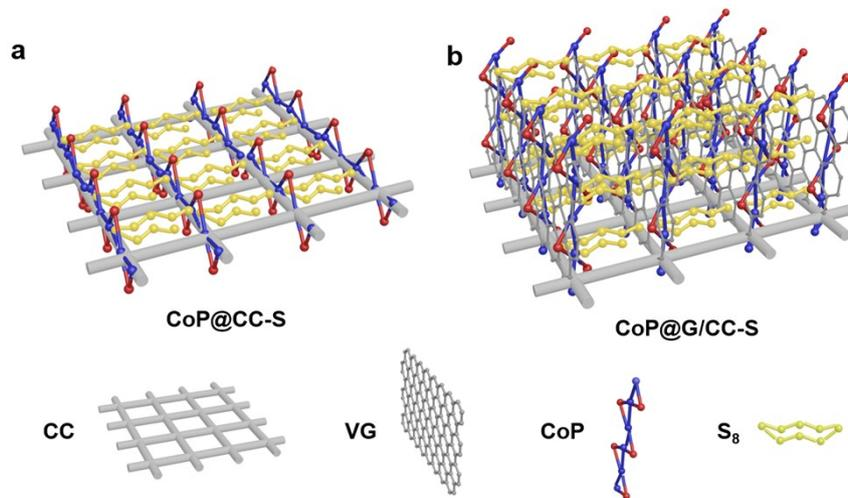
**Fig. S18.** Schematic illustration of the sulfur distribution at the CoP@CC and CoP@G/CC.
