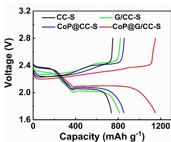
Fig. S11. Galvanostatic charge/discharge profiles of different cathodes at 0.5 C.
