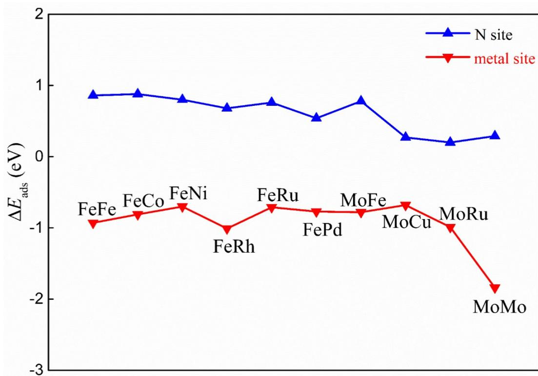
**Fig. S8.** The computed adsorption energies of H\* on N and metal sites of various BACs@NPG.
