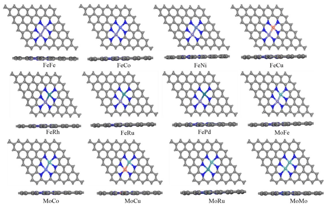
**Fig. S1.** The optimized configurations of metal dimers embedded into N-doped porous graphene. Both top and side views were provided.
