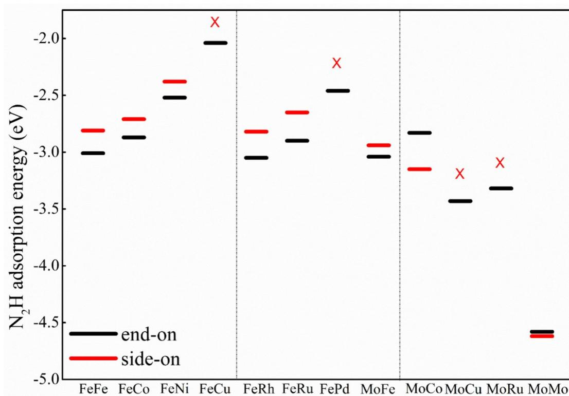
**Fig. S5.** The computed adsorption energies of  $N_2H^*$  species on various BACs@NPG via end-on and side-on patterns. X represents the unstable adsorption configurations.
