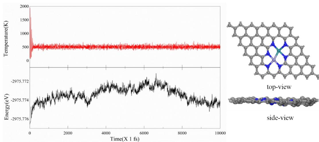
**Fig. S10.** Variations of temperature and energy against time for MD simulations of the FeRh@NPG, and the insets show top and side views of the snapshot of the atomic configuration. The simulation is run at 500 K for 10 ps with a time step of 1 fs.
