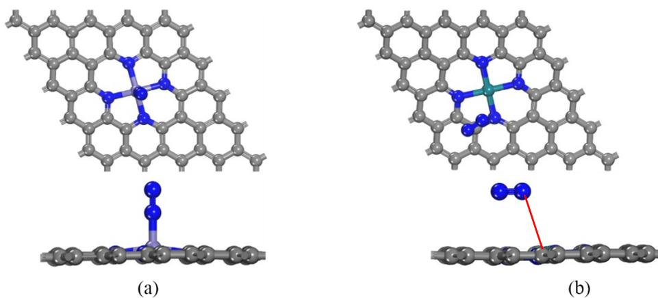
**Fig. S9.** The optimized adsorption configurations of N<sub>2</sub> molecule on single (a) Fe and (b) Rh atom supported on N-doped graphene.
