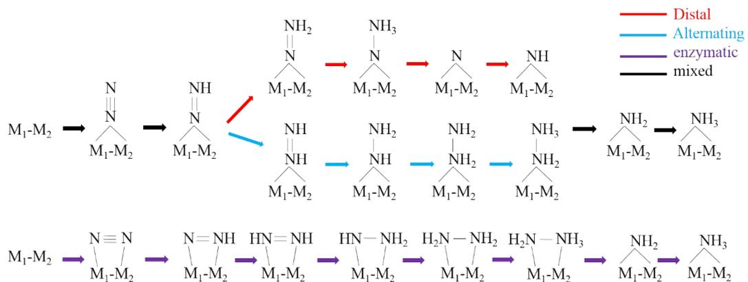
**Scheme S1.** The possible reaction mechanisms for eNRR on DACs@NPG
