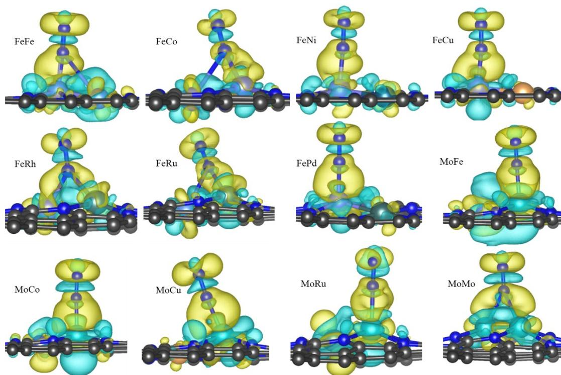
**Fig. S4.** The differential charge density distribution of  $N_2$  molecule adsorbed on these BACs@NPG at isosurfaces of  $\pm 0.01 \text{ e}/\text{\AA}^3$ . The charge accumulation and depletion are denoted by cyan and yellow colors, respectively.
