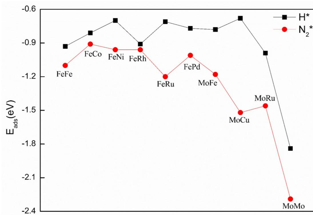
**Fig. S7.** The computed adsorption energies of  $H^*$  and  $N_2^*$  on BACs@NPG.
