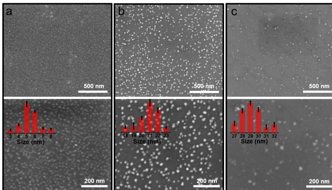
**Fig. S2** FESEM images of a) 100 cycles Ni, b) 400 cycles Ni, and c) 600 cycles Ni deposited on silicon wafers.
