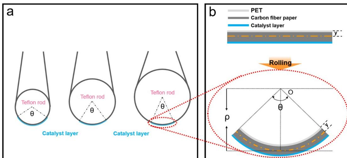
**Fig. S18** Schematic illustration of the structure of (a) Co-NCF@600-Ni/CFP belt rolling onto 10-mm, 20-mm and 30-mm rods and (b) the enlarged details of the rolled catalytic region of Co-NCF@600-Ni/CFP belt.
