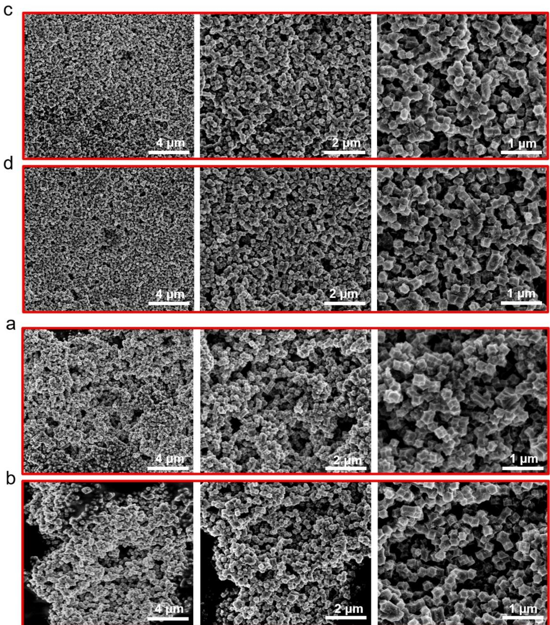
**Fig. S1** FESEM images of a) Co-NCF, b) Co-NCF@100-Ni, c) Co-NCF@400-Ni, and d) Co-NCF@600-Ni.
