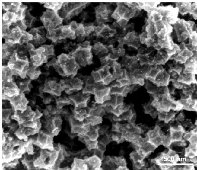
**Fig. S14** SEM image of Co-NCF@600-Ni after 20 h chronoamperometric test.
