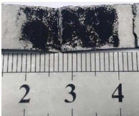
**Fig. S20** Digital photo of the Co-NCF@Ni/CFP electrode after 50 times of rolling and several times of electrochemical tests.
