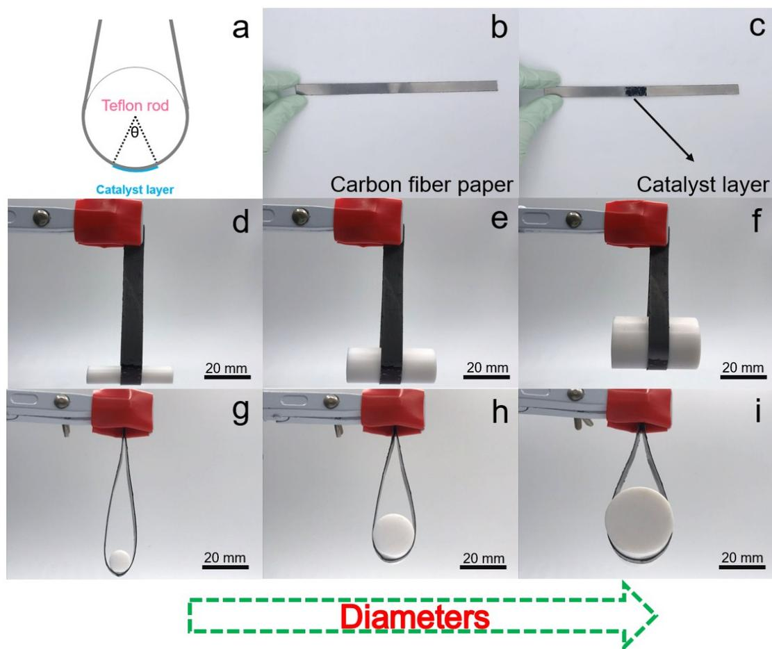
**Fig. S17** (a) Schematic illustration of the structure of Co-NCF@600-Ni/CFP electrode. Digital photos of (b) CFP and (c) Co-NCF@600-Ni/CFP belt. (d-f) Front view photos and (g-i) lateral view photos of Co-NCF@600-Ni/CFP rolling onto (d, g) 10-mm Teflon rod, (e, h) 20-mm Teflon rod, and (f, i) 30-mm Teflon rod.
