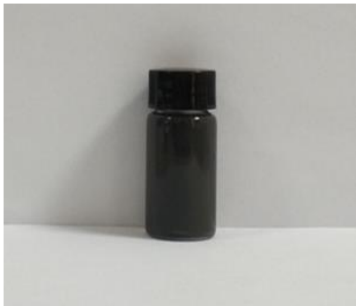
Figure S11. Optical photo of graphene nanosheet dispersion. The concentration of the graphene nanosheet dispersion is 0.529 mg/mL. Graphene nanosheet dispersion is a black homogeneous dispersion solution with no obvious precipitation.
